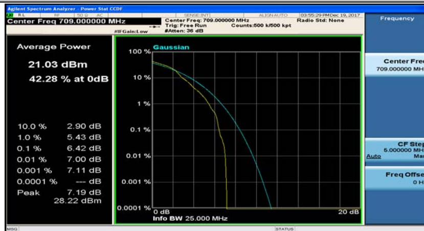
Channel Bandwidth: 10 MHz_LCH_16QAM_25RB#0
