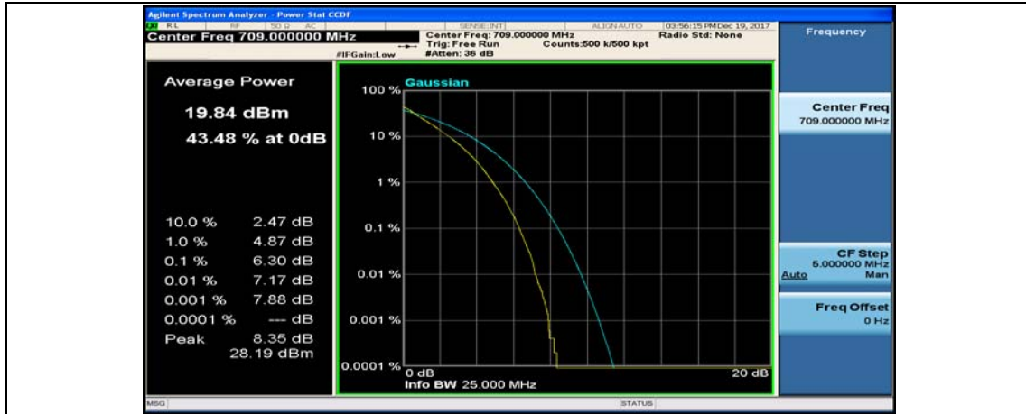
Channel Bandwidth: 10 MHz_MCH_QPSK_1RB#0
