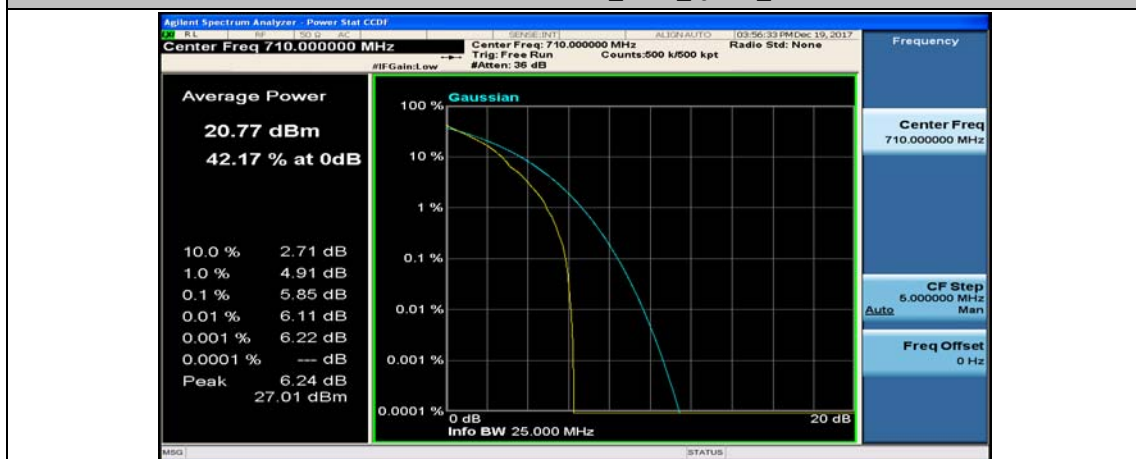
Channel Bandwidth: 10 MHz_MCH_QPSK_1RB#24
