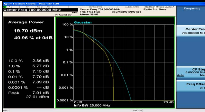
Channel Bandwidth: 10 MHz_LCH_16QAM_1RB#49
