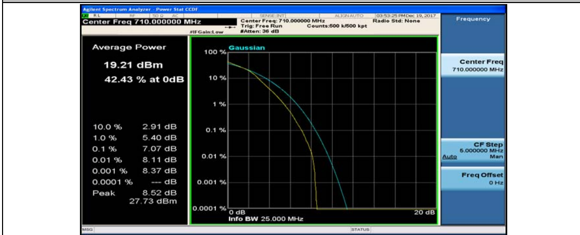
(Channel Bandwidth: 5 MHz)_MCH_16QAM_25RB#0
