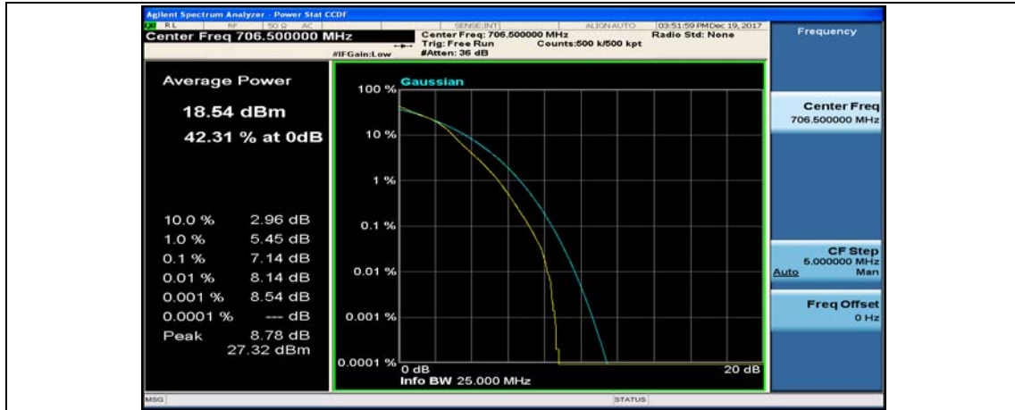
(Channel Bandwidth: 5 MHz)_MCH_16QAM_1RB#0
