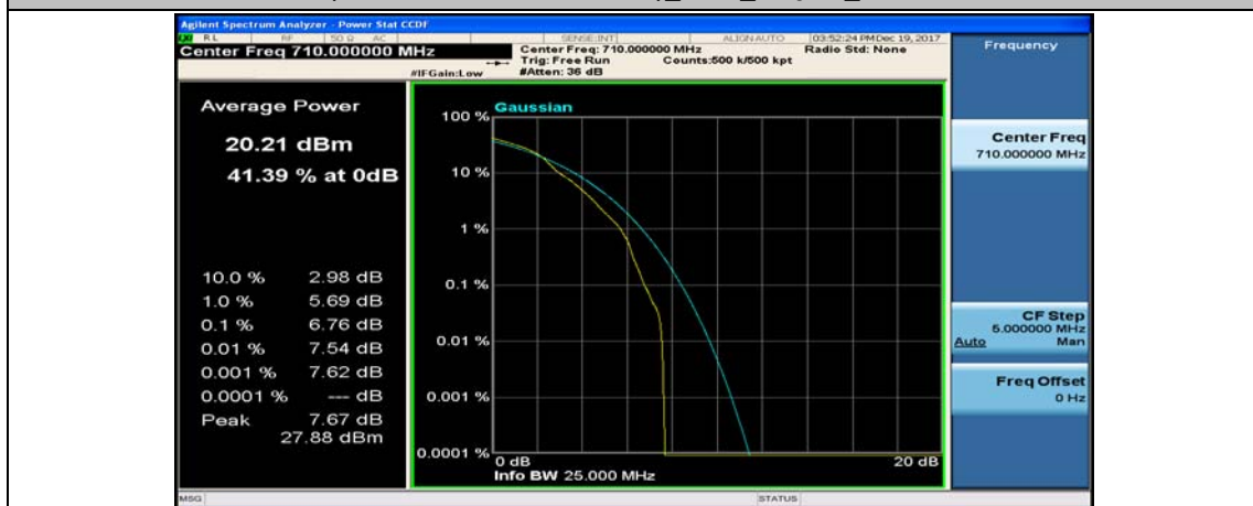
(Channel Bandwidth: 5 MHz)_MCH_16QAM_1RB#12
