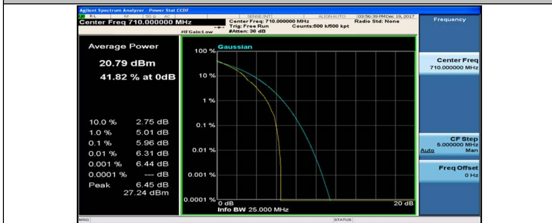
Channel Bandwidth: 10 MHz_MCH_QPSK_1RB#49
