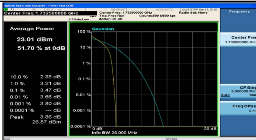
(Channel Bandwidth:15 MHz)_MCH_QPSK_37RB#38
