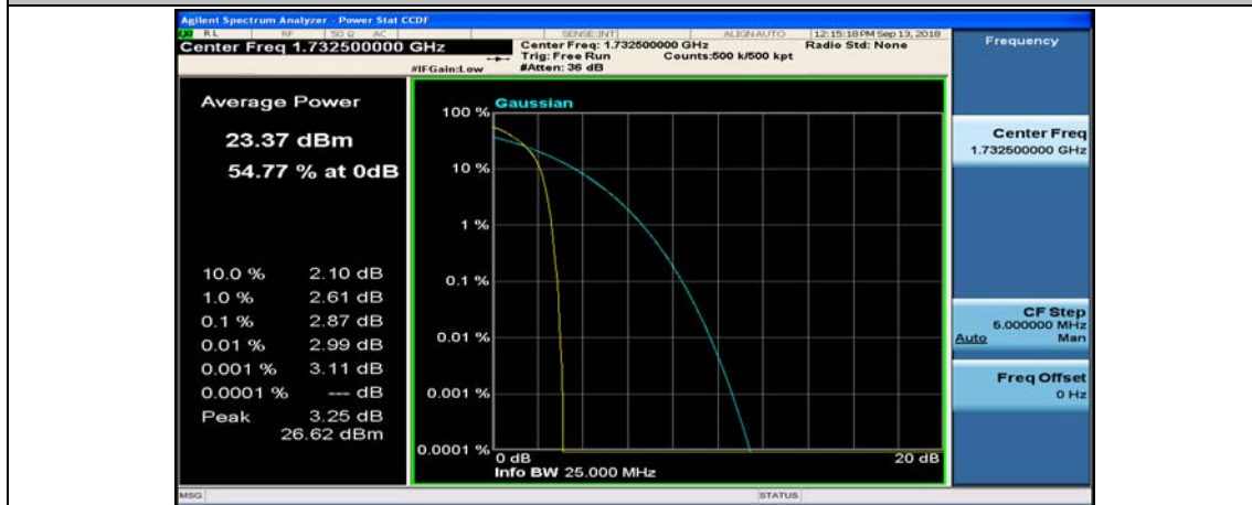
(Channel Bandwidth:15 MHz)_MCH_QPSK_1RB#74
