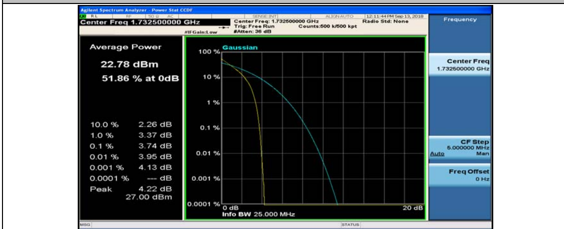
Channel Bandwidth: 10 MHz_MCH_QPSK_50RB#0
