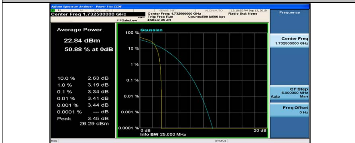
Channel Bandwidth: 10 MHz_MCH_16QAM_1RB#49
