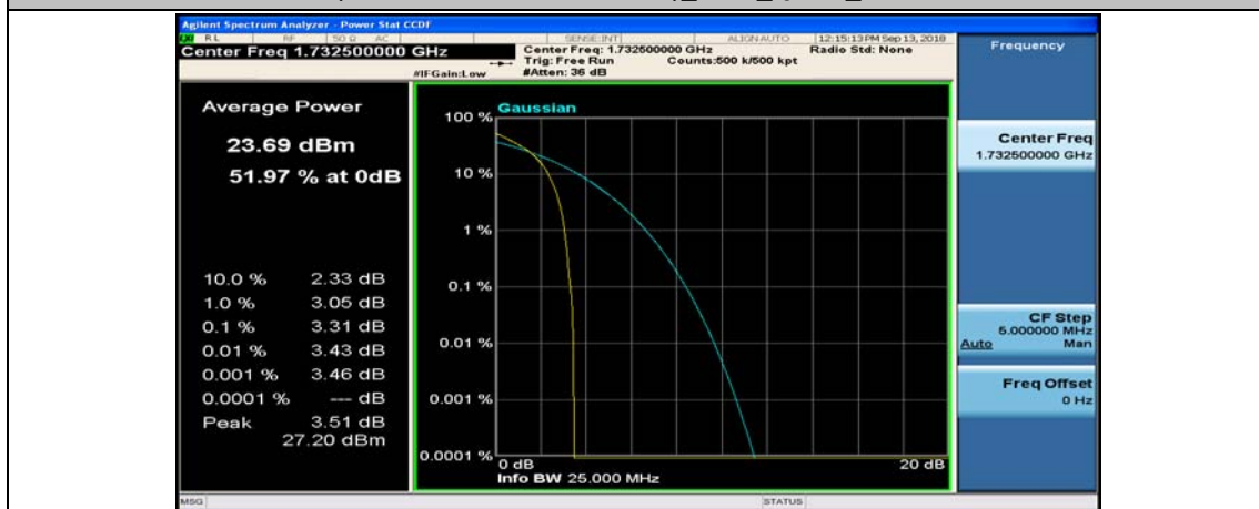
(Channel Bandwidth:15 MHz)_MCH_QPSK_1RB#37
