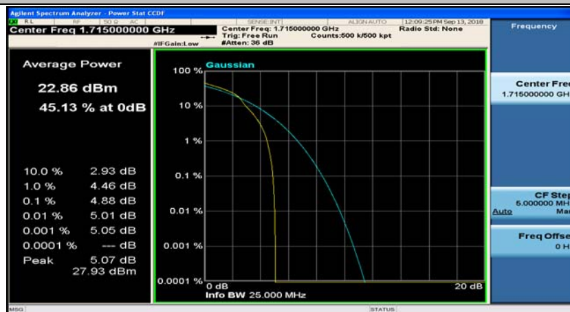
Channel Bandwidth: 10 MHz_LCH_16QAM_25RB#0
