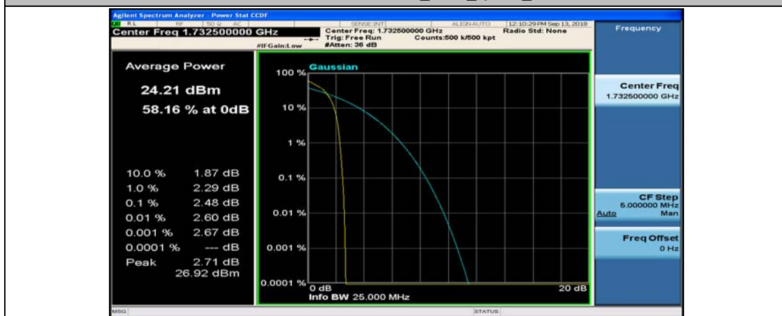
Channel Bandwidth: 10 MHz_MCH_QPSK_1RB#24
