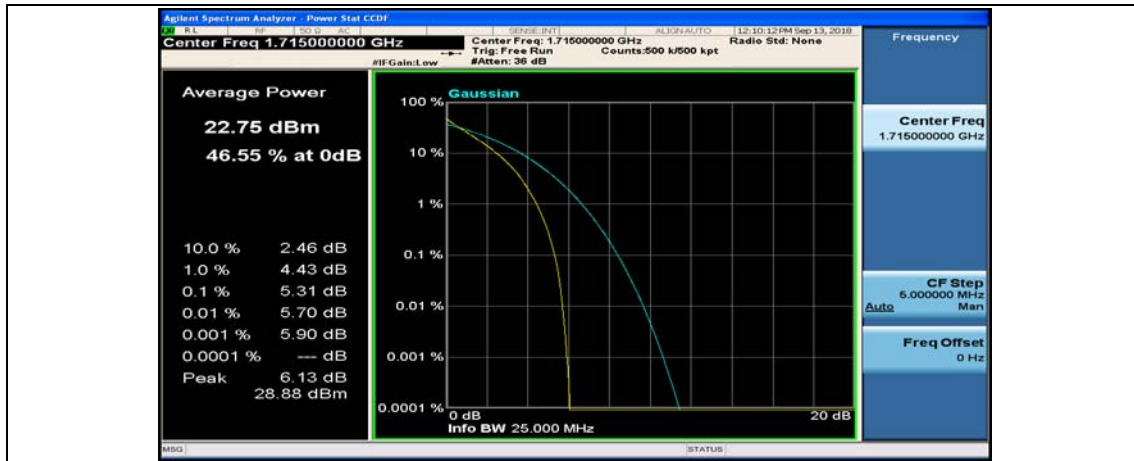
Channel Bandwidth: 10 MHz_MCH_QPSK_1RB#0
