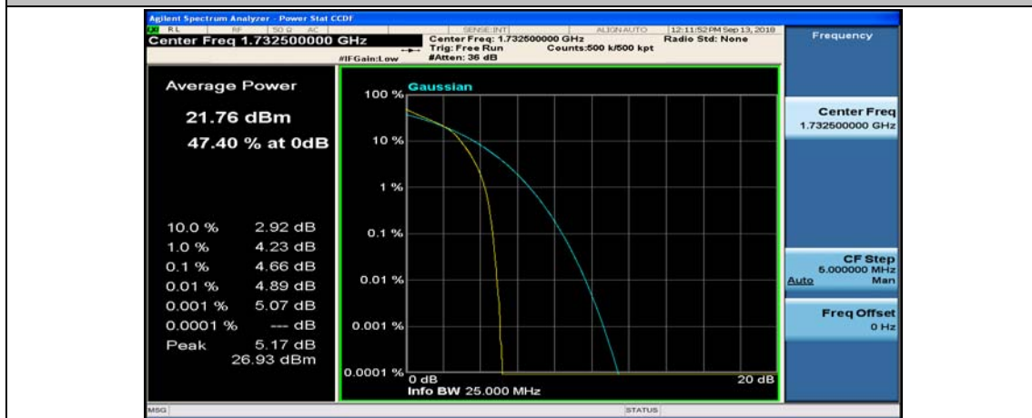
Channel Bandwidth: 10 MHz_MCH_16QAM_50RB#0
