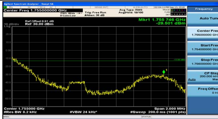
(Channel Bandwidth: 1.4 MHz)_HCH_16QAM_1RB#3
