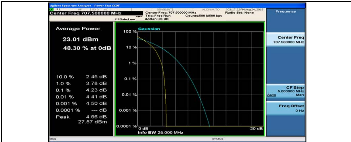
(Channel Bandwidth: 5 MHz)_MCH_QPSK_25RB#0
