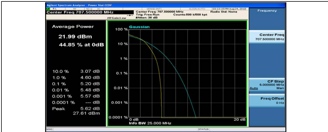
(Channel Bandwidth: 3 MHz)_MCH_16QAM_15RB#0
