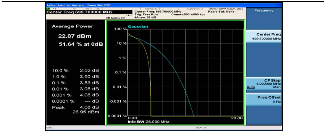
(Channel Bandwidth: 1.4 MHz)_MCH_QPSK_1RB#0
