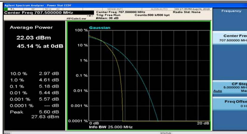
(Channel Bandwidth: 5 MHz)_MCH_16QAM_12RB#13
