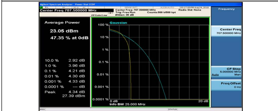
(Channel Bandwidth: 5 MHz)_MCH_16QAM_1RB#24
