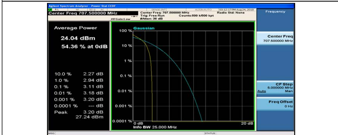
(Channel Bandwidth: 3 MHz)_MCH_QPSK_1RB#14
