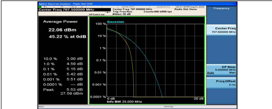
(Channel Bandwidth: 5 MHz)_MCH_16QAM_25RB#0
