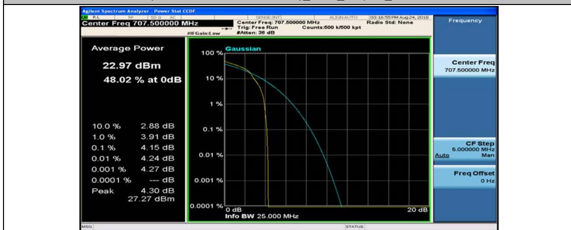
(Channel Bandwidth: 5 MHz)_MCH_16QAM_1RB#12
