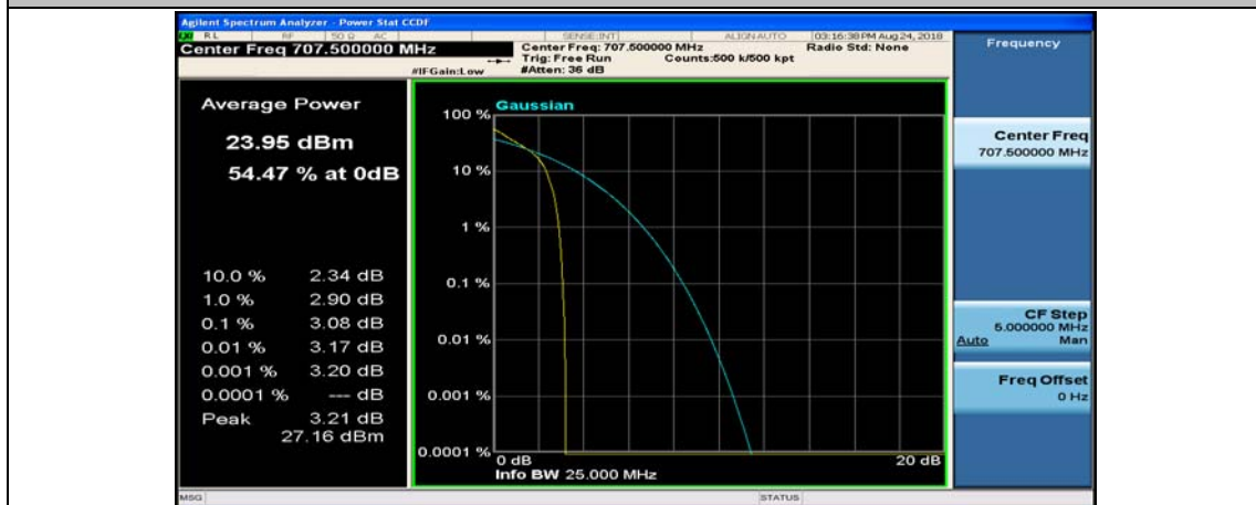
(Channel Bandwidth: 5 MHz)_MCH_QPSK_1RB#12
