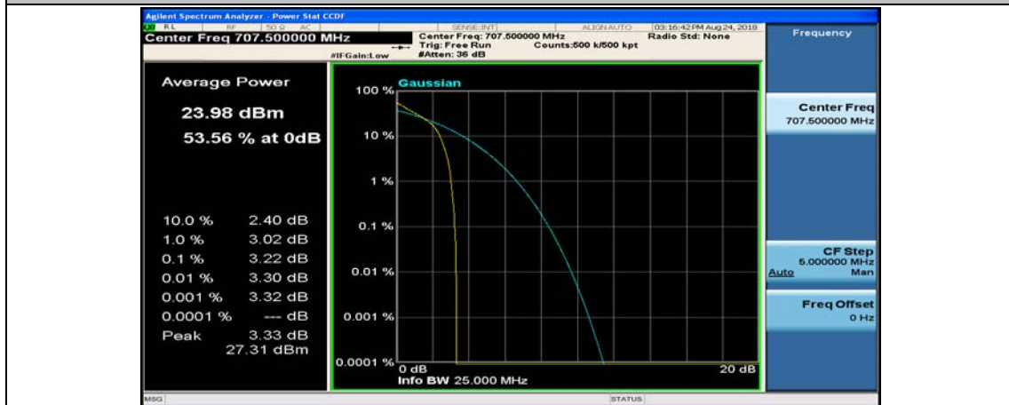
(Channel Bandwidth: 5 MHz)_MCH_QPSK_1RB#24
