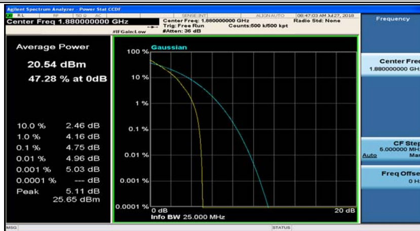
Channel Bandwidth: 10 MHz_MCH_QPSK_25RB#12
