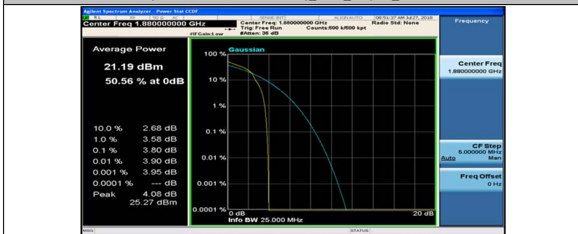
(Channel Bandwidth:15 MHz)_MCH_16QAM_1RB#37
