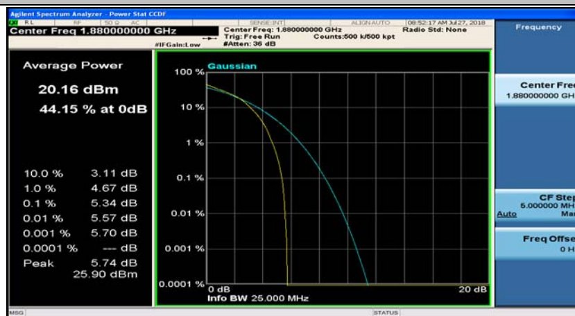
(Channel Bandwidth:15 MHz)_MCH_16QAM_37RB#18
