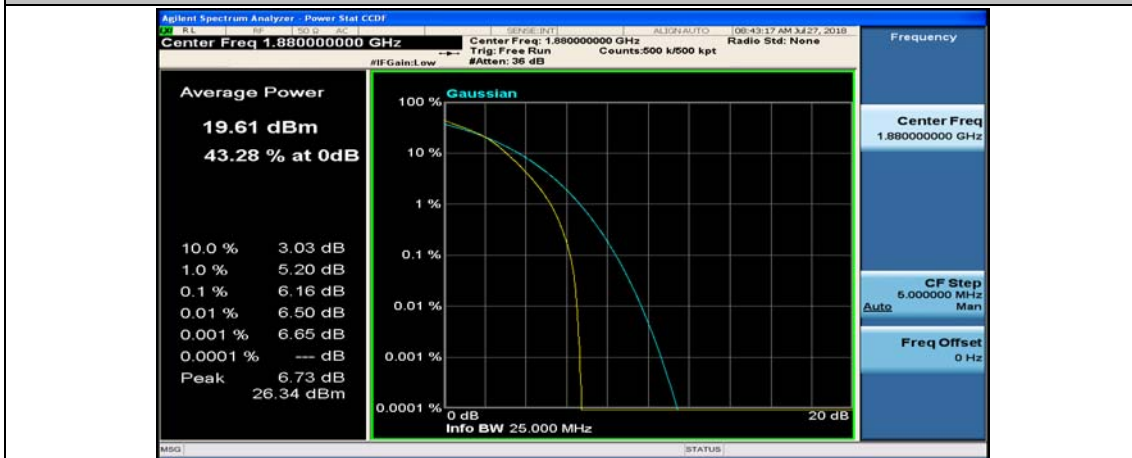
(Channel Bandwidth: 5 MHz)_MCH_16QAM_25RB#0
