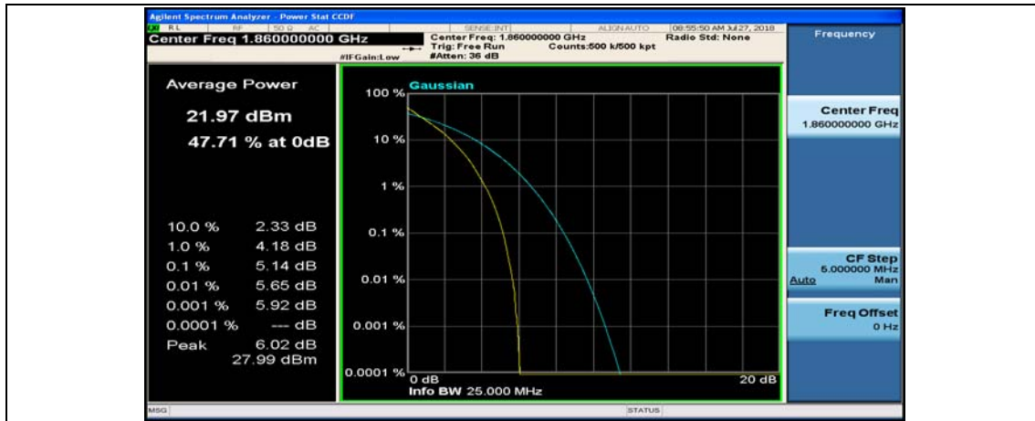
(Channel Bandwidth:20 MHz)_MCH_QPSK_1RB#0
