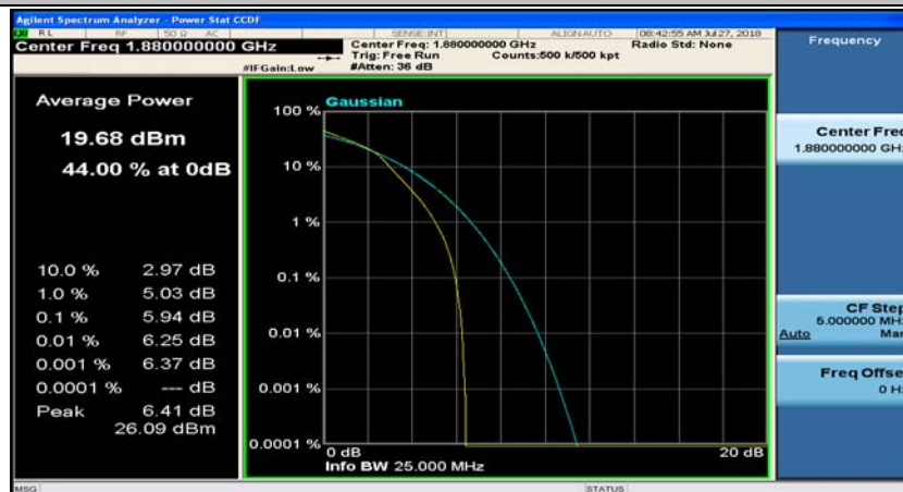
(Channel Bandwidth: 5 MHz)_MCH_16QAM_12RB#13
