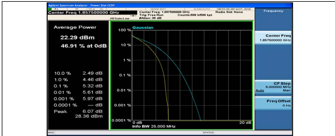
(Channel Bandwidth:15 MHz)_MCH_QPSK_1RB#0
