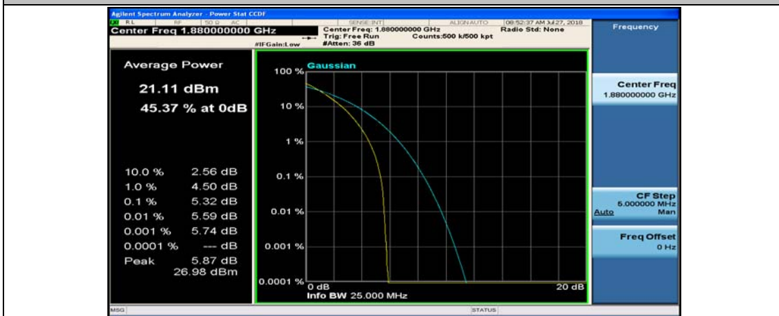
(Channel Bandwidth:15 MHz)_MCH_QPSK_75RB#0
