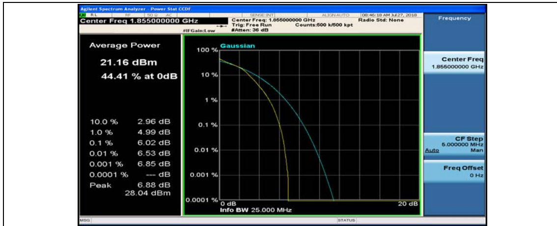
Channel Bandwidth: 10 MHz_MCH_16QAM_1RB#0
