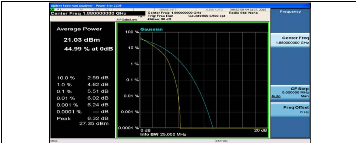
(Channel Bandwidth:15 MHz)_MCH_QPSK_75RB#0
