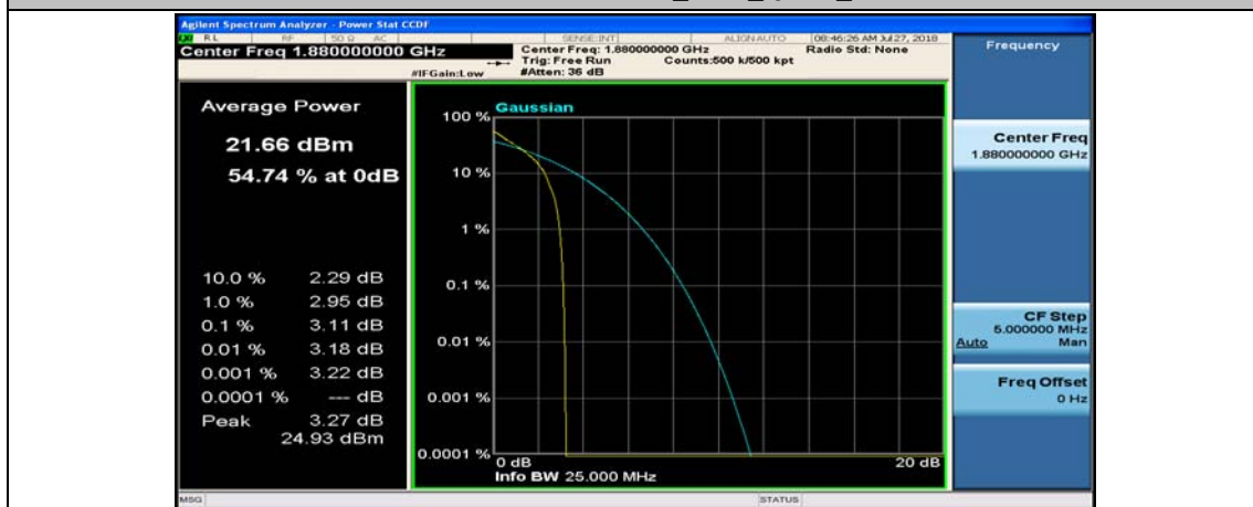
Channel Bandwidth: 10 MHz_MCH_QPSK_1RB#24
