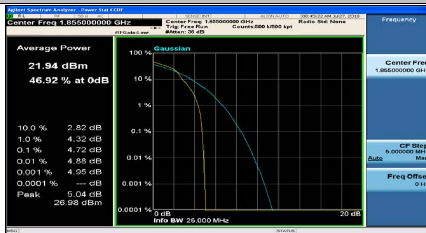
Channel Bandwidth: 10 MHz_LCH_16QAM_25RB#0
