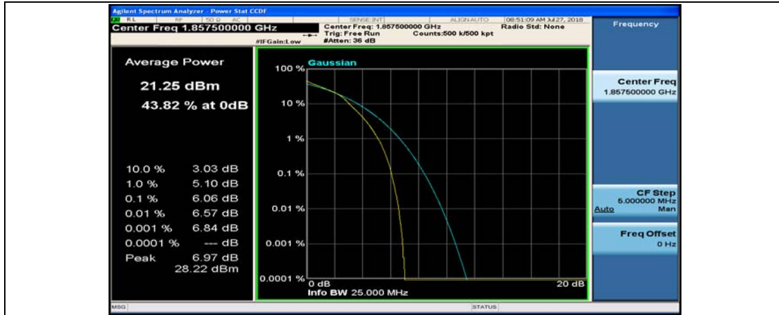
(Channel Bandwidth:15 MHz)_MCH_16QAM_1RB#0
