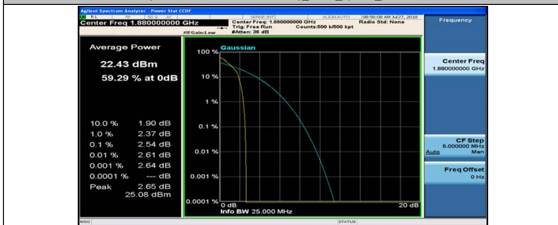
(Channel Bandwidth:20 MHz)_MCH_QPSK_1RB#49
