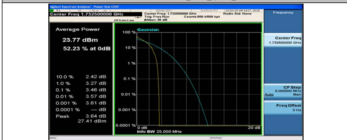
Channel Bandwidth: 10 MHz_MCH_QPSK_1RB#24
