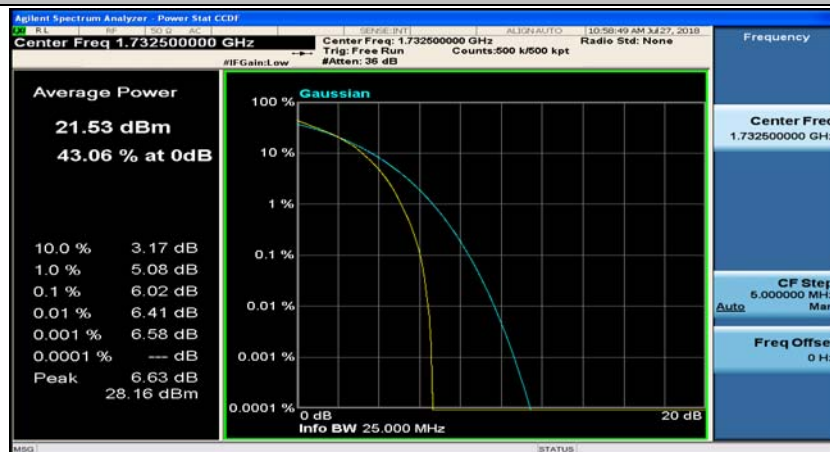
(Channel Bandwidth:15 MHz)_MCH_16QAM_37RB#38
