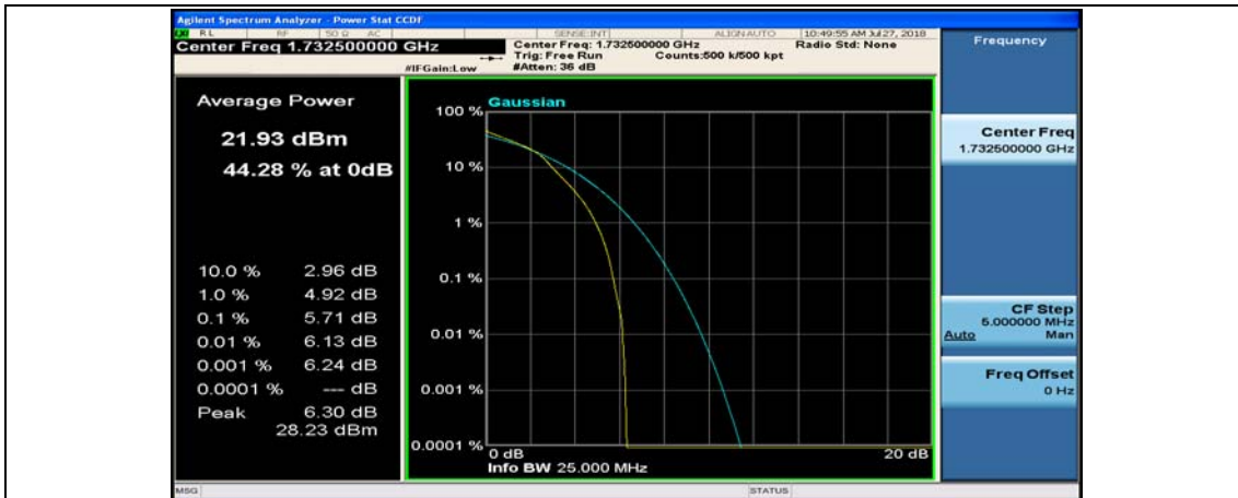
(Channel Bandwidth: 5 MHz)_MCH_16QAM_25RB#0
