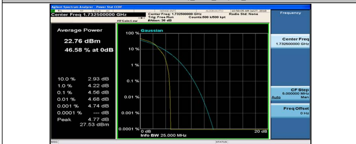
(Channel Bandwidth:15 MHz)_MCH_16QAM_1RB#37
