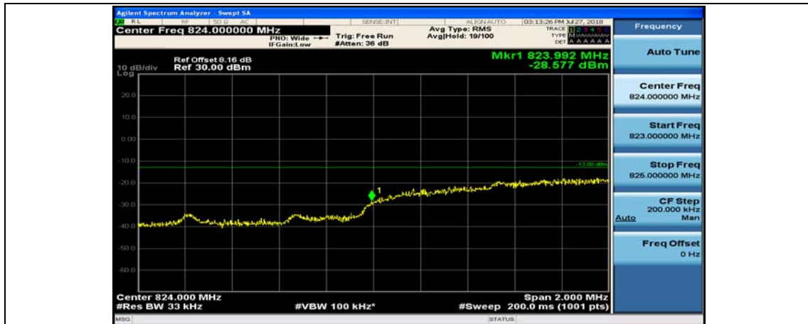
(Channel Bandwidth: 3 MHz)_LCH_QPSK_15RB#0
