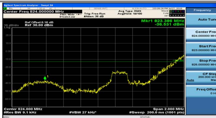
(Channel Bandwidth: 1.4 MHz)_LCH_QPSK_1RB#5
