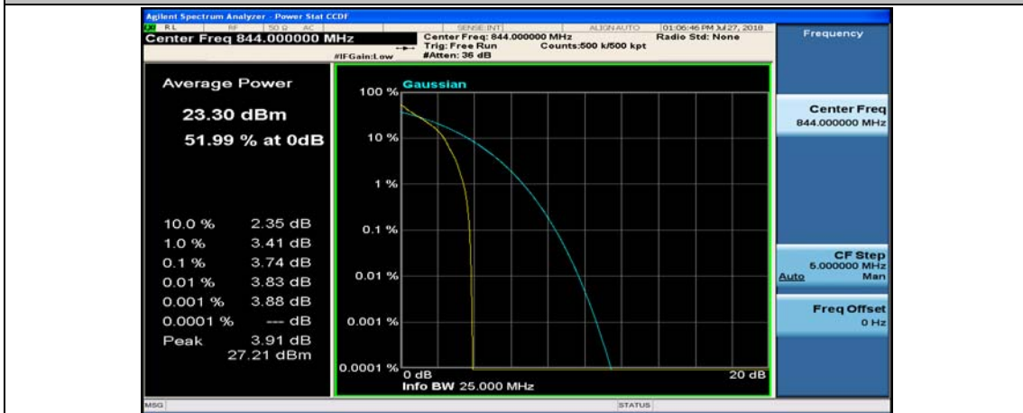
Channel Bandwidth: 10 MHz_HCH_QPSK_1RB#24
