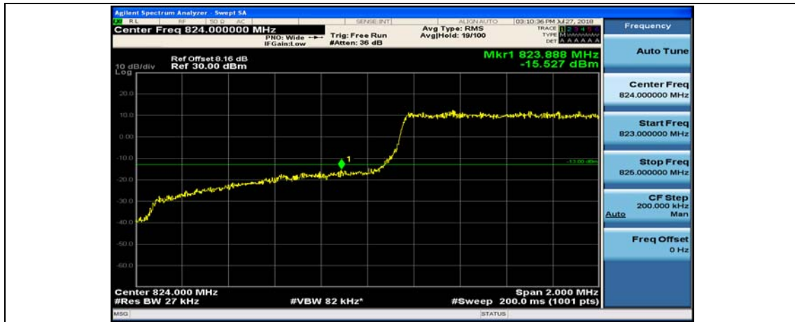
(Channel Bandwidth: 1.4 MHz)_HCH_QPSK_1RB#0
