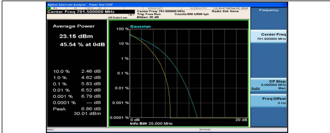
(Channel Bandwidth: 5 MHz)_MCH_QPSK_1RB#0
