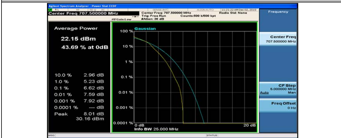
(Channel Bandwidth: 5 MHz)_MCH_16QAM_25RB#0
