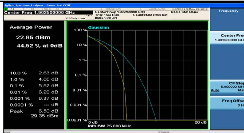
(Channel Bandwidth:15 MHz)_HCH_QPSK_37RB#18
