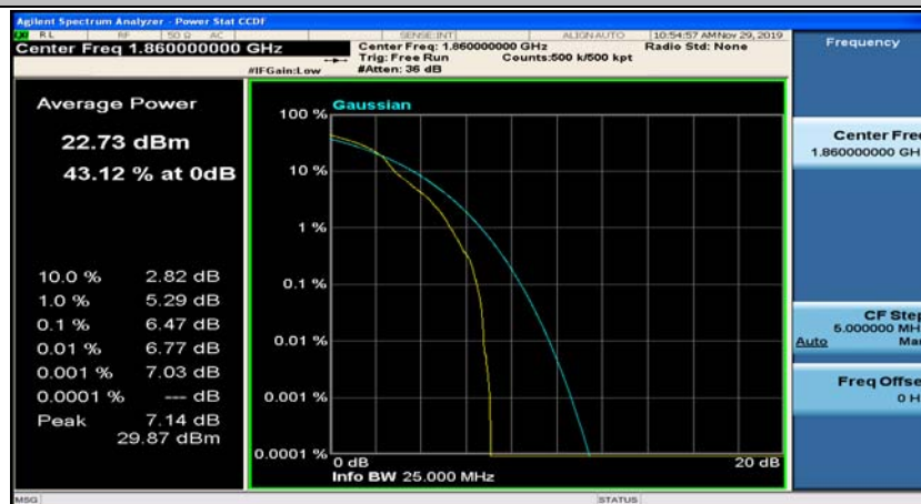
(Channel Bandwidth:20 MHz)_LCH_16QAM_50RB#0
