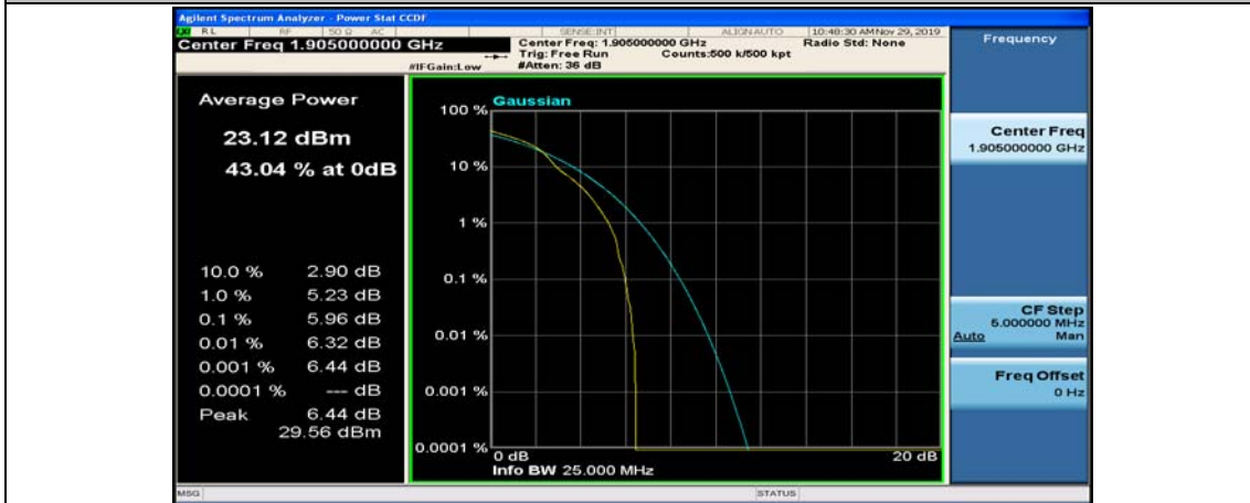
Channel Bandwidth: 10 MHz_HCH_16QAM_1RB#24
