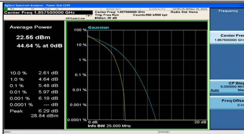
(Channel Bandwidth:15 MHz)_LCH_QPSK_37RB#38
