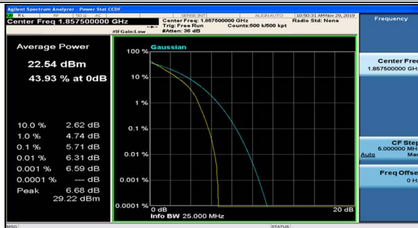
(Channel Bandwidth:15 MHz)_LCH_QPSK_75RB#0
