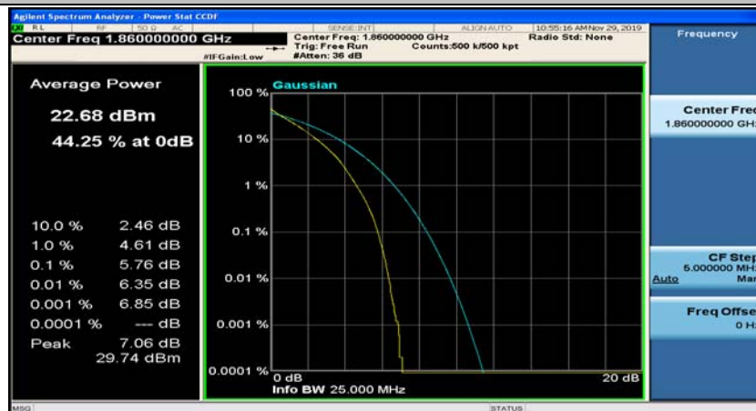
(Channel Bandwidth:20 MHz)_LCH_QPSK_100RB#0
