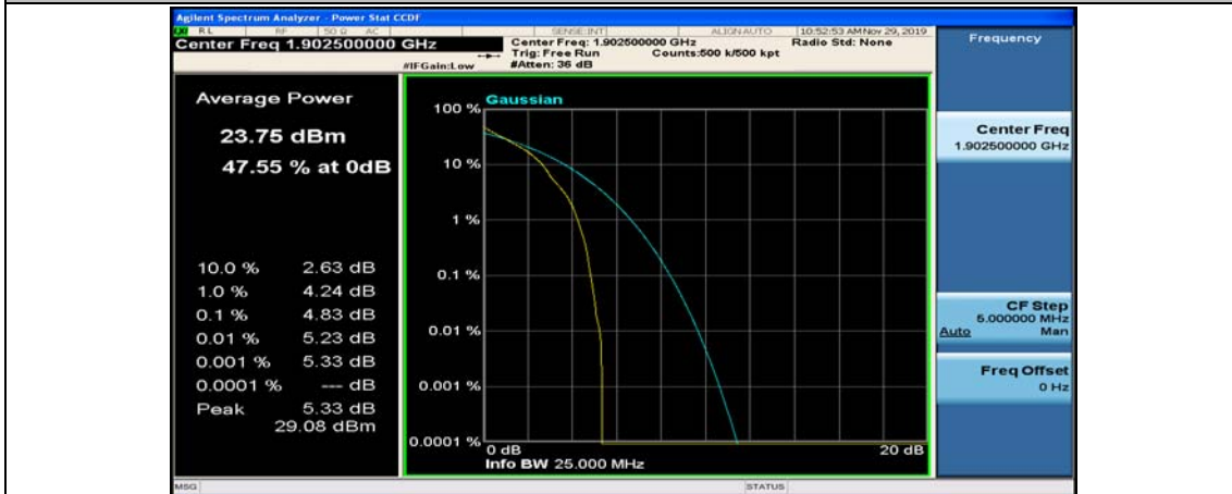
(Channel Bandwidth:15 MHz)_HCH_QPSK_1RB#37
