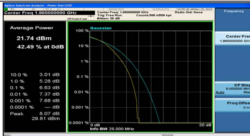
(Channel Bandwidth:20 MHz)_LCH_16QAM_100RB#0
