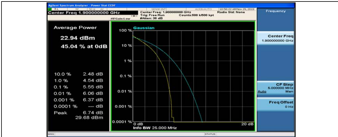
(Channel Bandwidth:20 MHz)_HCH_QPSK_50RB#50
