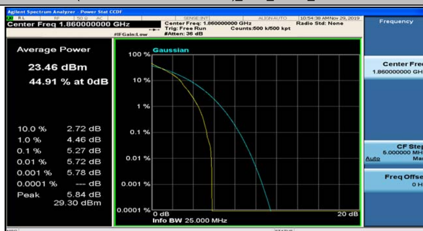
(Channel Bandwidth:20 MHz)_LCH_QPSK_50RB#0
