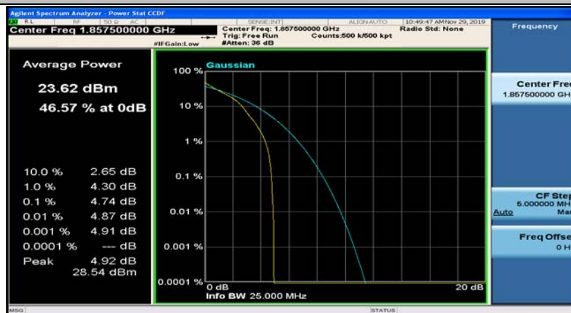
(Channel Bandwidth:15 MHz)_LCH_QPSK_1RB#74
