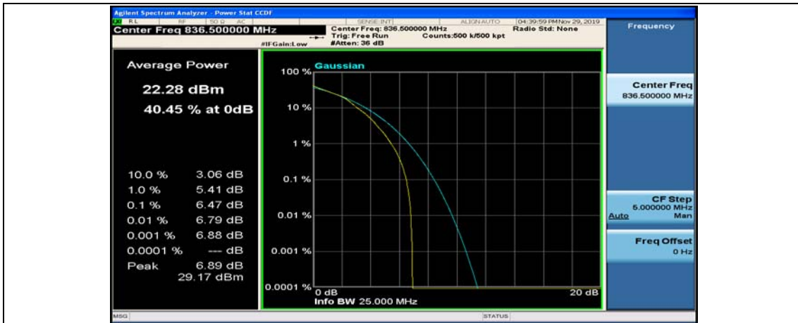
(Channel Bandwidth: 1.4 MHz)_MCH_16QAM_6RB#0
