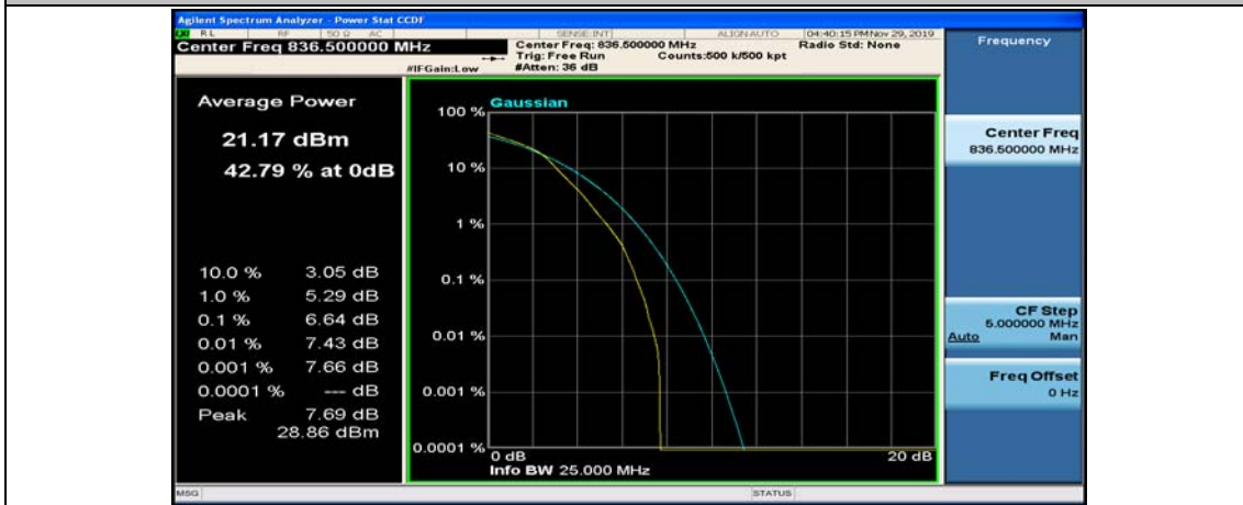
(Channel Bandwidth: 1.4 MHz)_MCH_16QAM_6RB#0
