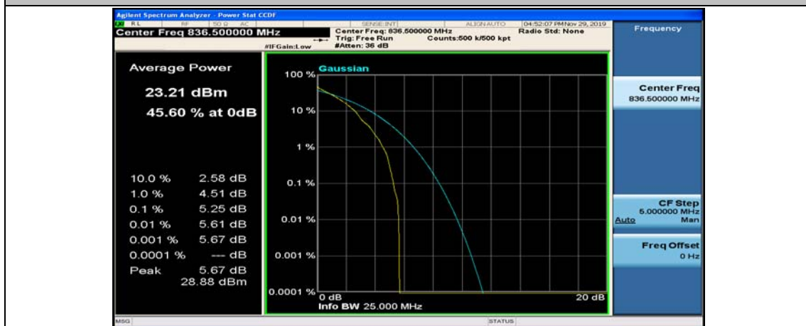
Channel Bandwidth: 10 MHz_MCH_QPSK_1RB#49
