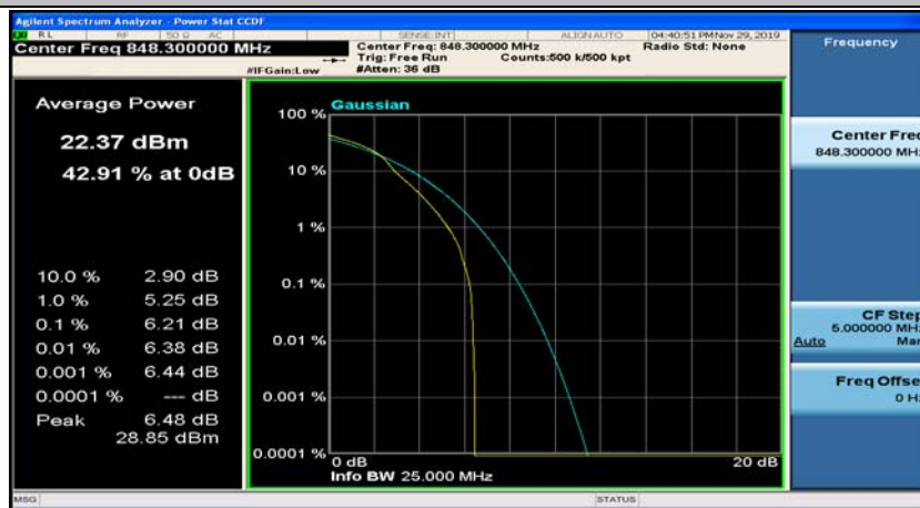
(Channel Bandwidth: 1.4 MHz)_HCH_16QAM_3RB#0
