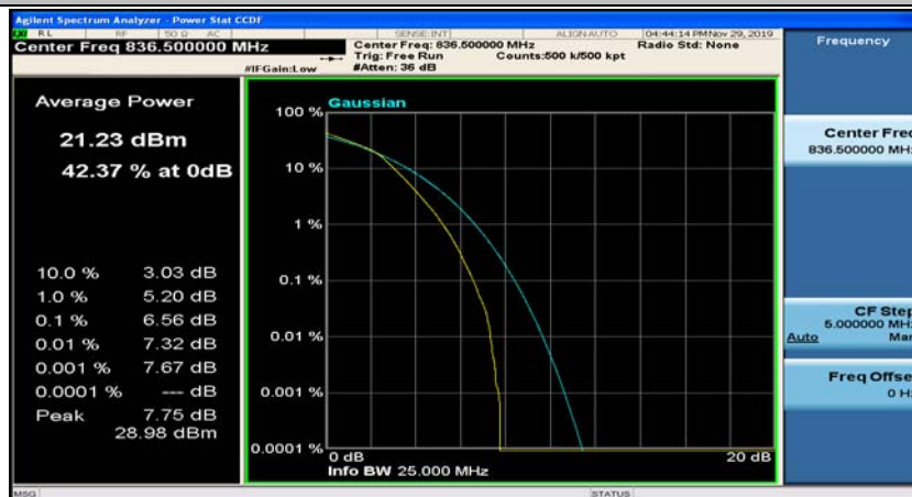
(Channel Bandwidth: 3 MHz)_MCH_16QAM_8RB#7
