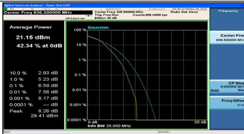
(Channel Bandwidth: 5 MHz)_MCH_16QAM_12RB#6
