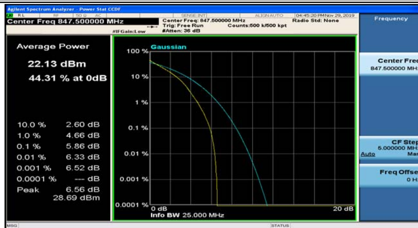
(Channel Bandwidth: 3 MHz)_HCH_QPSK_8RB#4
