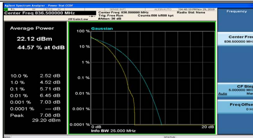
(Channel Bandwidth: 5 MHz)_MCH_QPSK_12RB#13
