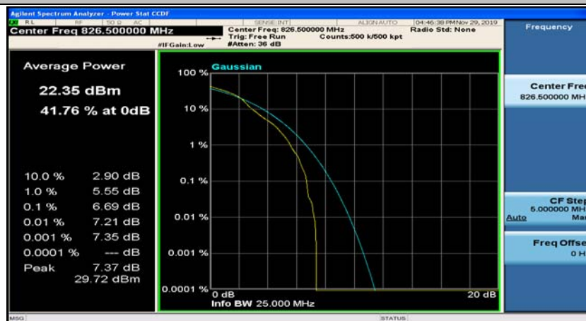
(Channel Bandwidth: 5 MHz)_LCH_16QAM_12RB#0
