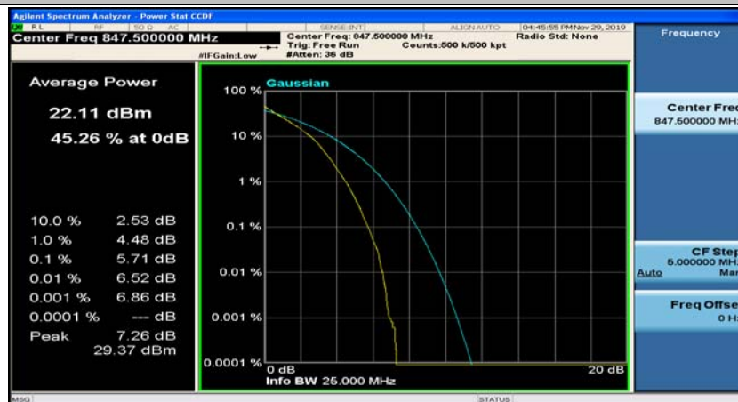
(Channel Bandwidth: 3 MHz)_HCH_QPSK_15RB#0
