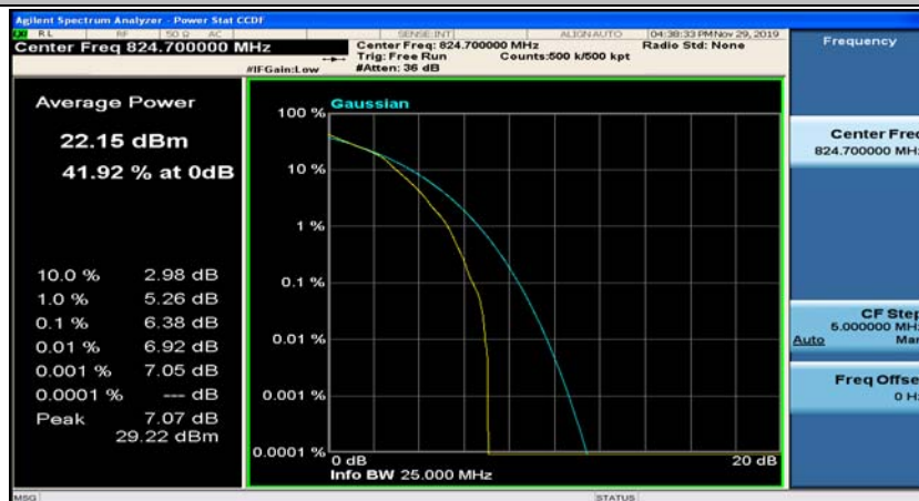
(Channel Bandwidth: 1.4 MHz)_LCH_16QAM_6RB#0
