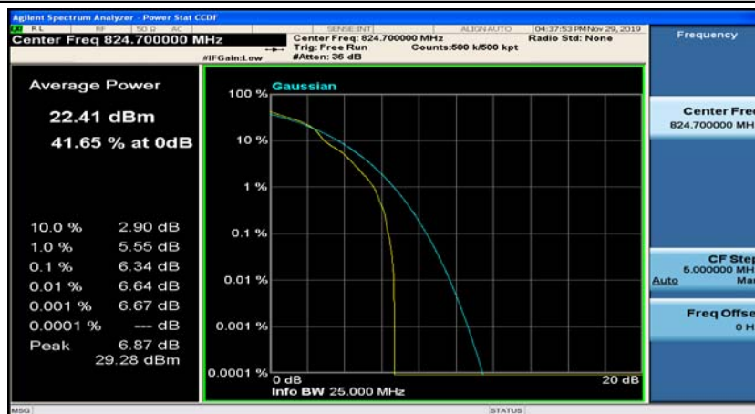
(Channel Bandwidth: 1.4 MHz)_LCH_16QAM_1RB#5
