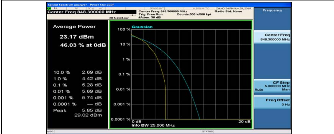
(Channel Bandwidth: 1.4 MHz)_HCH_QPSK_1RB#3
