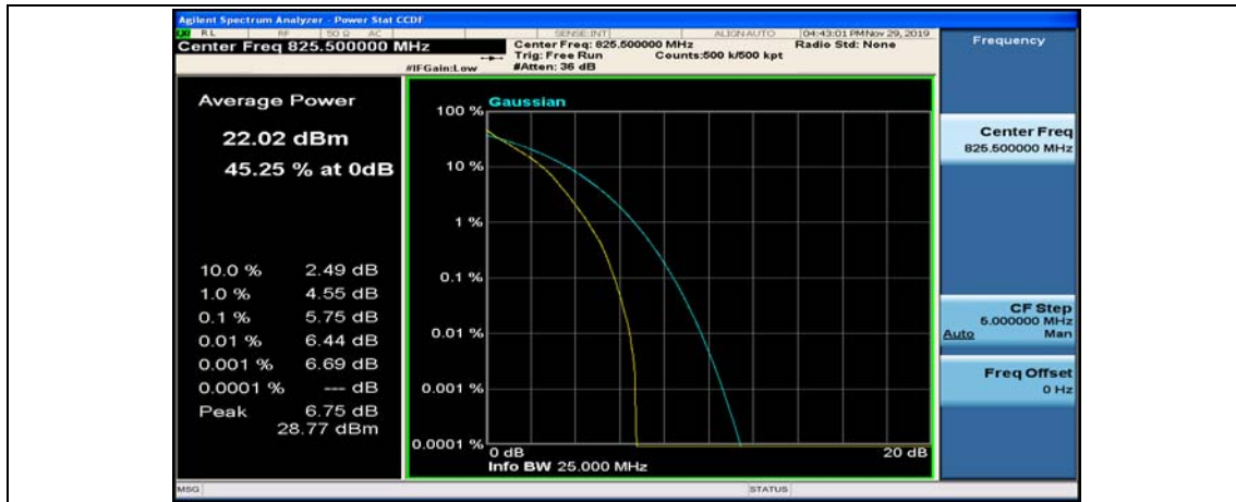
(Channel Bandwidth: 3 MHz)_MCH_QPSK_1RB#0
