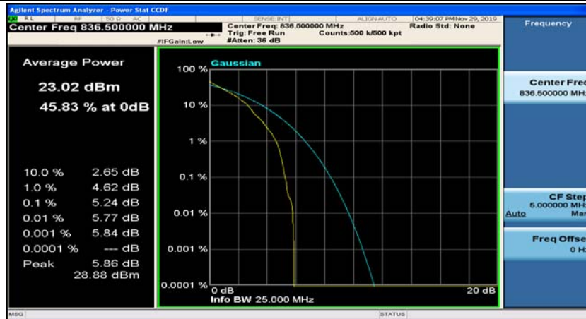
(Channel Bandwidth: 1.4 MHz)_MCH_QPSK_3RB#0
