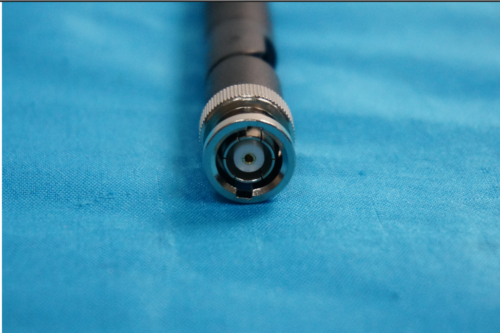
Antenna 2: AC-Q915I08 is Dipole antenna. Gain:5dBi
