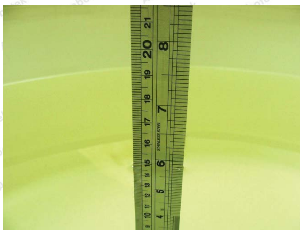
Photo of Liquid Height for Body SAR
