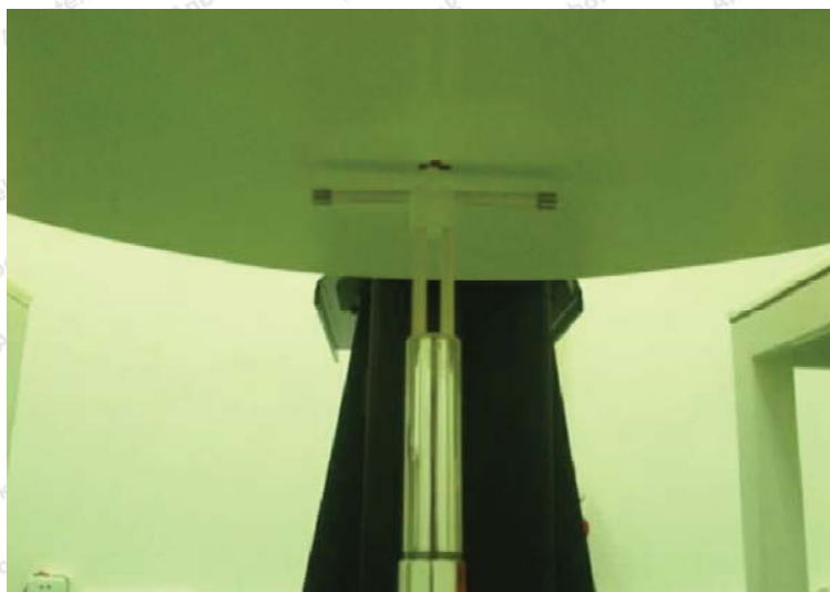
Photo of Dipole Setup
