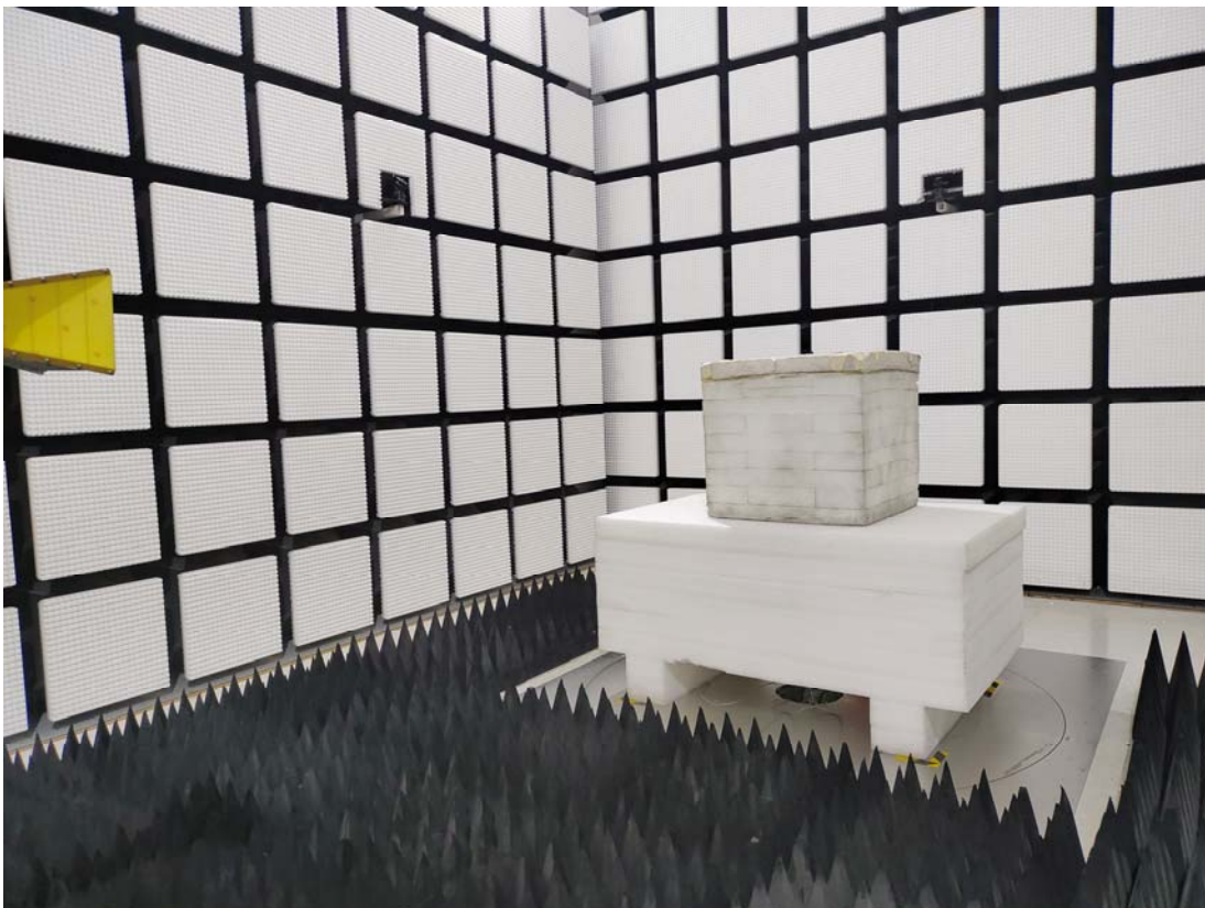
Radiated Emission Above 1GHz View
