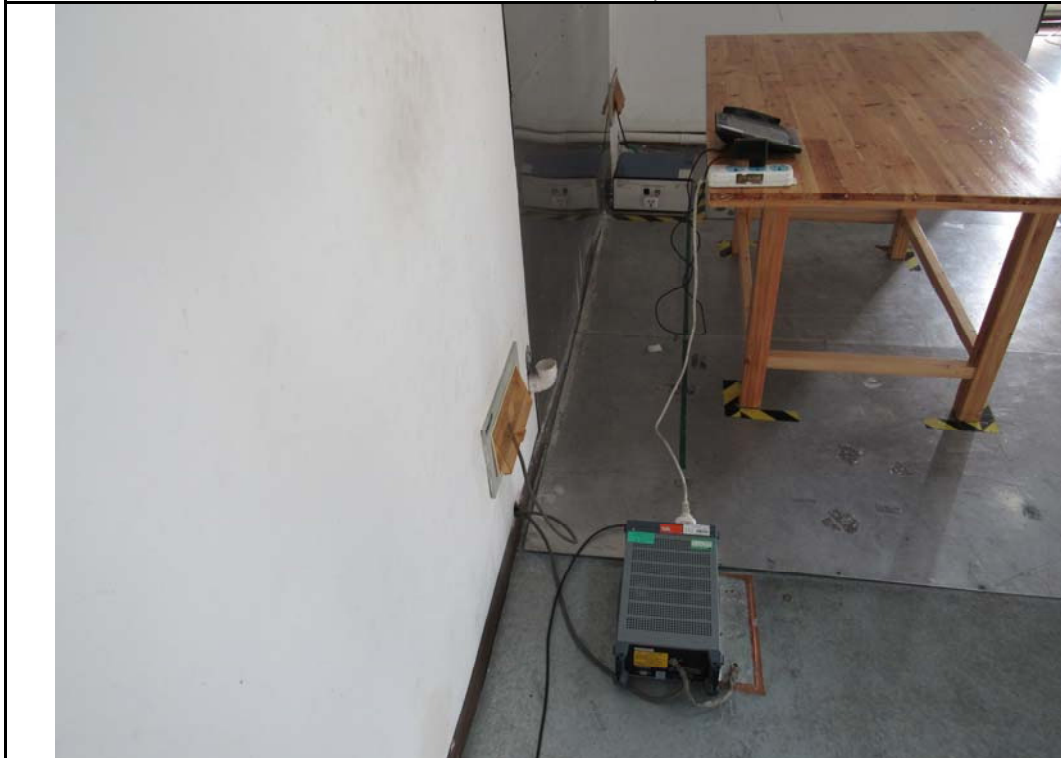
Conducted Emissions Test Setup Side View
