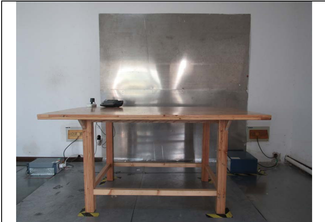
Conducted Emissions Test Setup Front View
