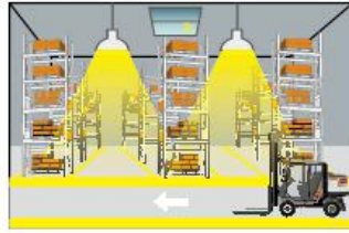
② Motion detected, lamp automatically lights up to 100%.
