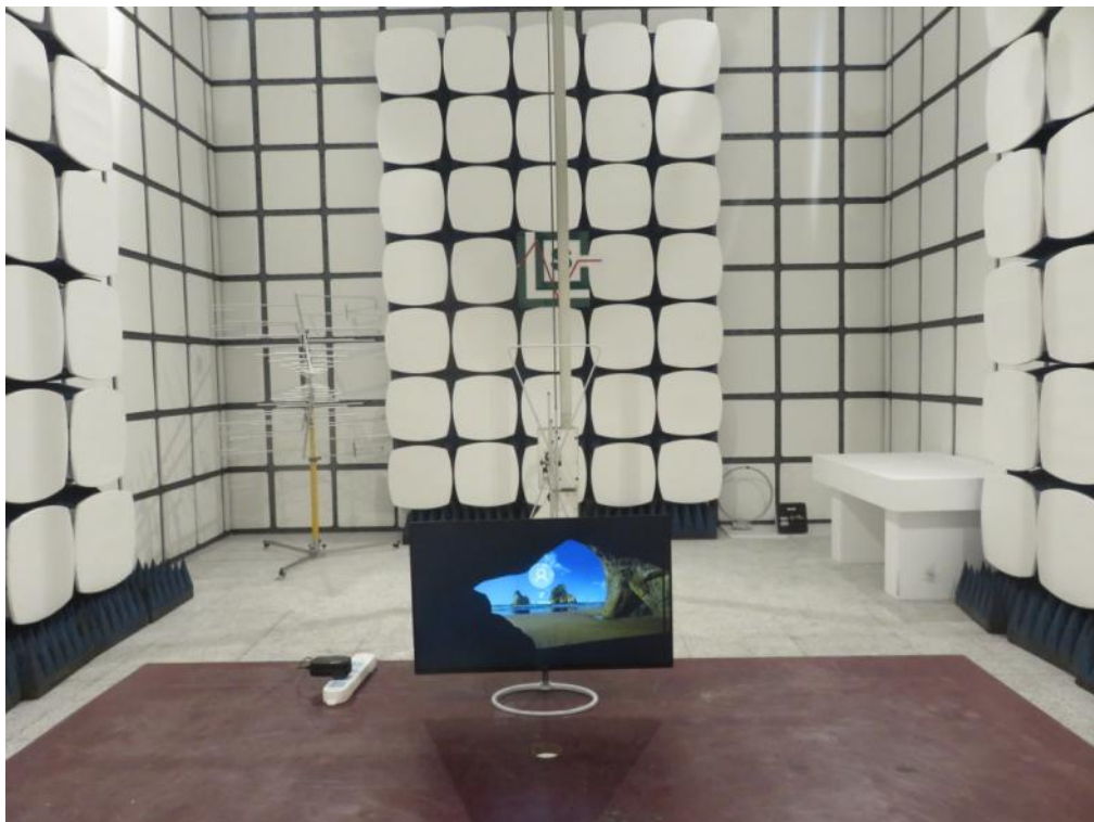
Radiated emission below 1GHz
