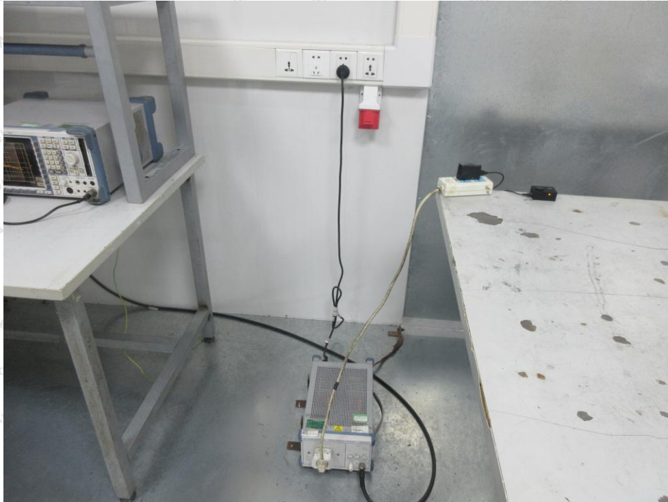
Photo of Conducted Emission Measurement
