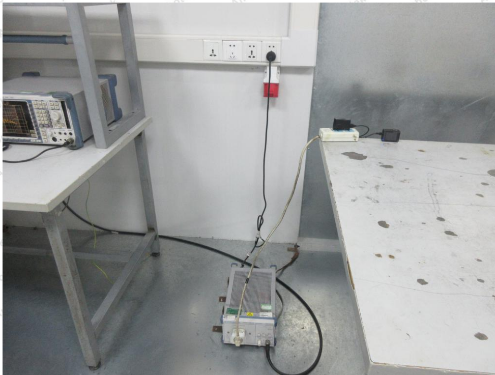
Photo of Conducted Emission Measurement
