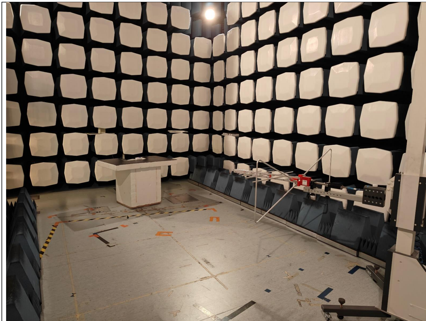
Picture 6, Radiated Spurious Emissions, common setup, TX 30 - 1000 MHz and RX 30 - 1000 MHz
