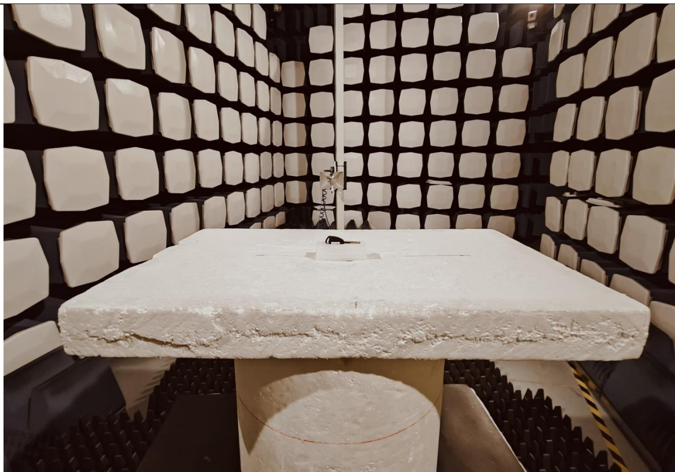
Picture 11, Radiated Spurious Emissions, EUT setup back, TX 1 – 18 GHz and RX 1 – 12,75 GHz
