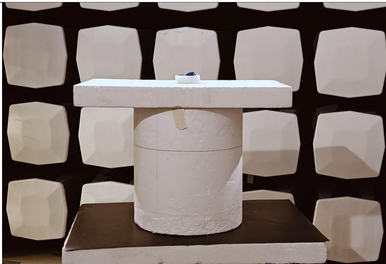
Picture 10, Radiated Spurious Emissions, EUT setup front, TX 1 – 18 GHz and RX 1 – 12,75 GHz
