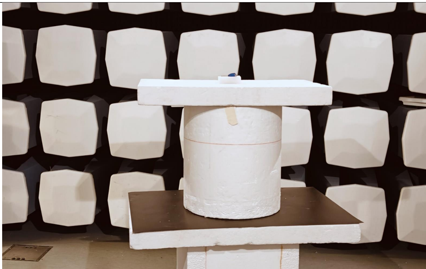
Picture 13, Radiated Spurious Emissions, EUT setup front, TX 18 – 26 GHz
