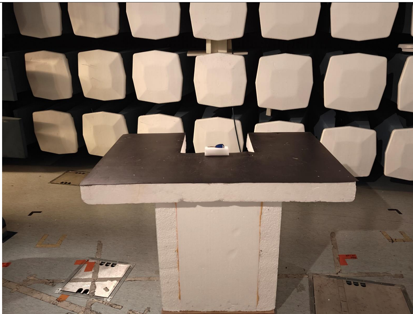
Picture 7, Radiated Spurious Emissions, EUT setup front, TX 30 - 1000 MHz and RX 30 - 1000 MHz
