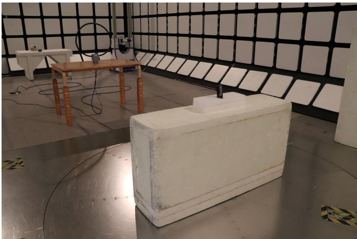
Photograph 3: Test setup for radiated tests (9 kHz – 30 MHz)
