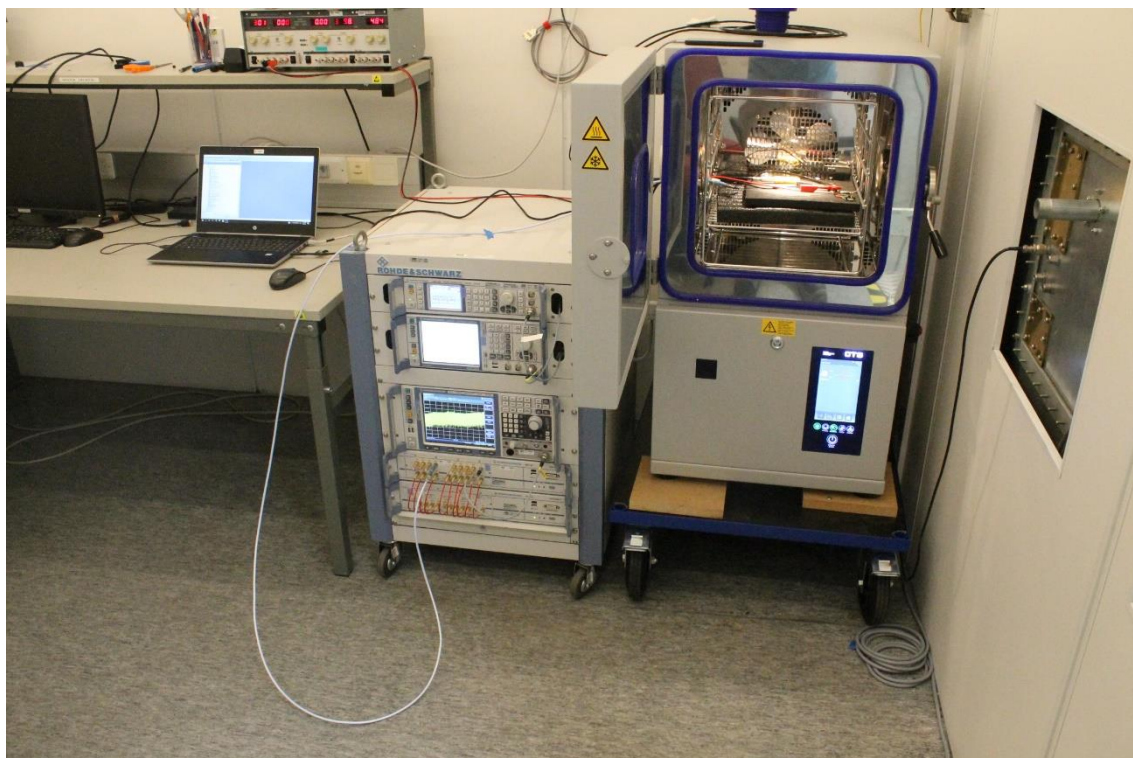
Photograph 1: Test setup for conducted tests
