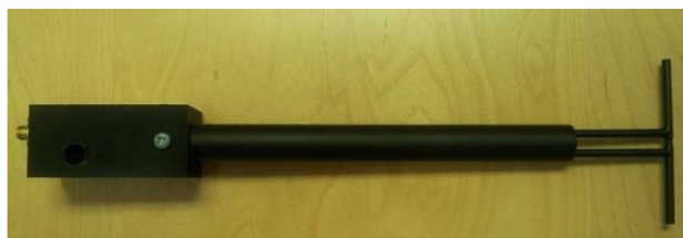
Figure 1 – MVG COMOSAR Validation Dipole
