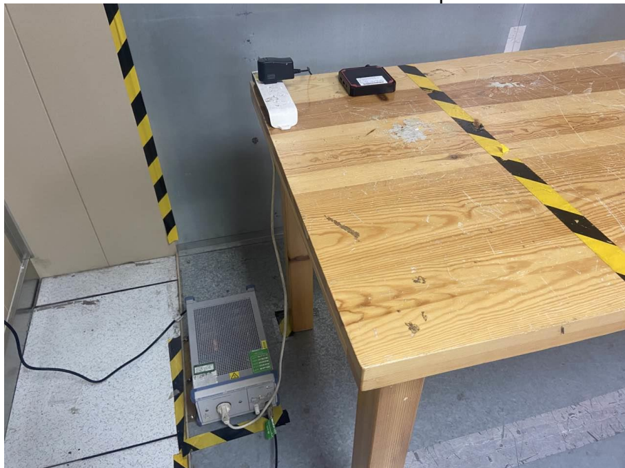
Conducted emission Test Setup
