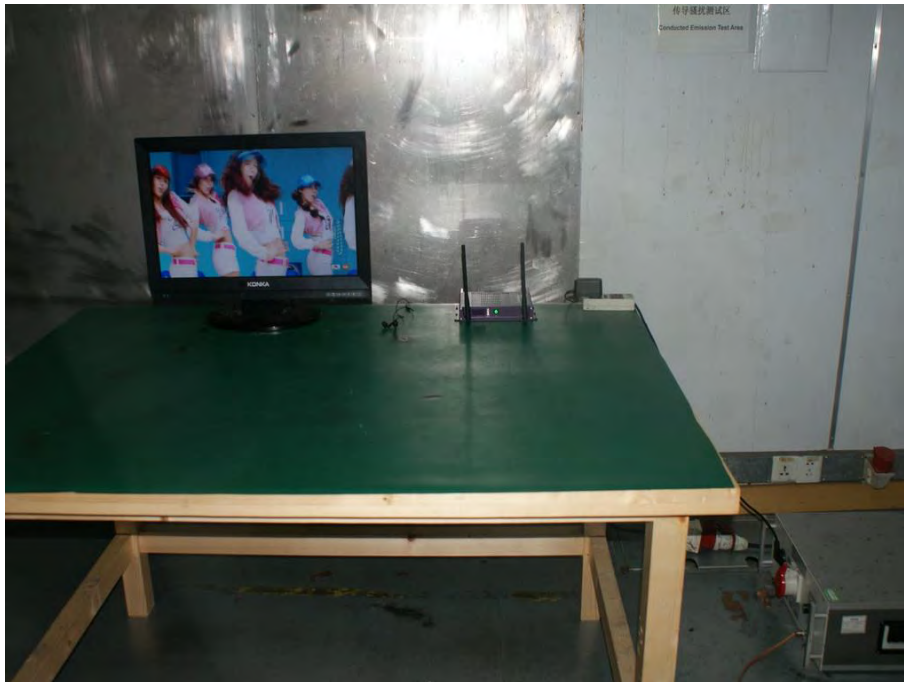
Photograph 5: Set-up for Conducted Emission on AC Mains
