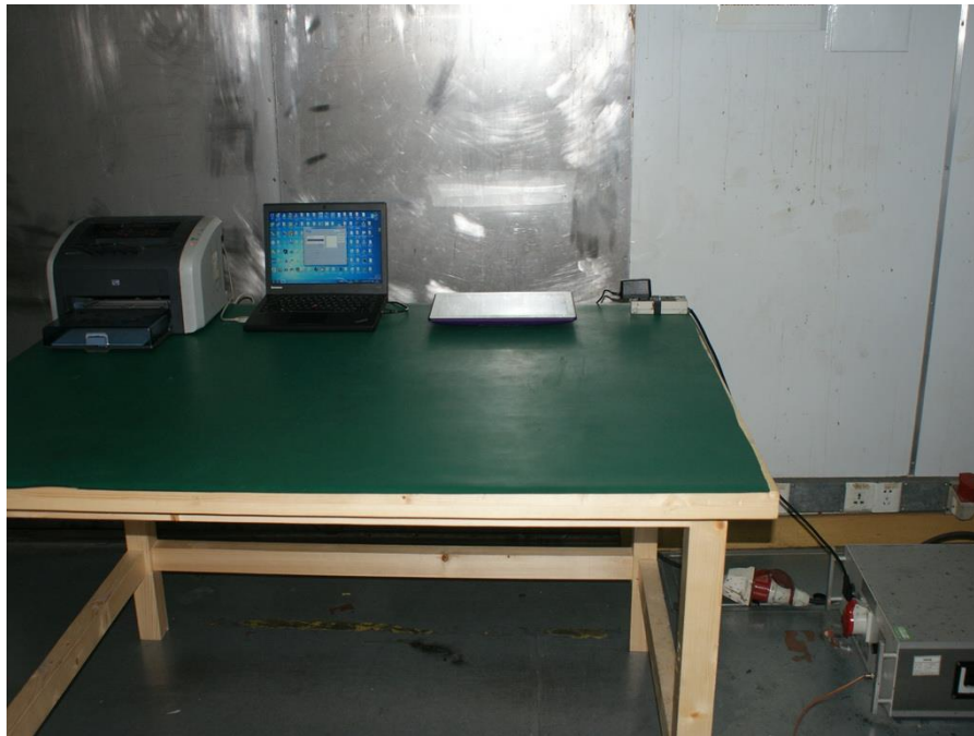
Photograph 2: Set-up for Radiated Emission (30MHz ~ 1GHz)
