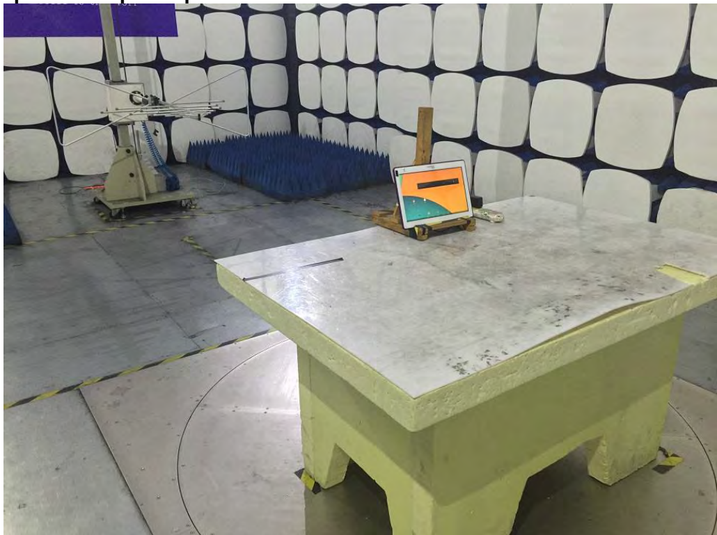
Photograph 2: Set-up for Spurious Emissions for 30 - 1000MHz
