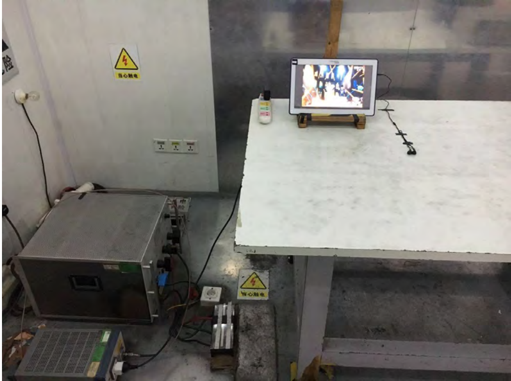
Photograph 2: Set-up for Spurious Emissions for 30 - 1000MHz
