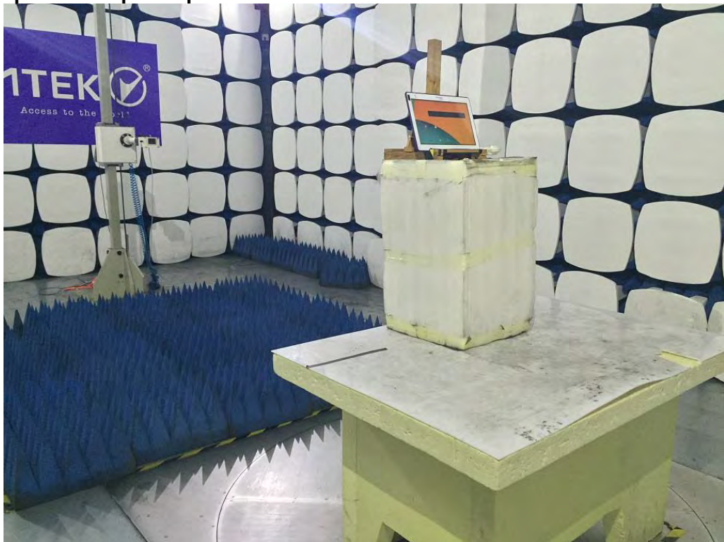
Photograph 4: Set-up for Spurious Emissions for 18 - 40GHz
