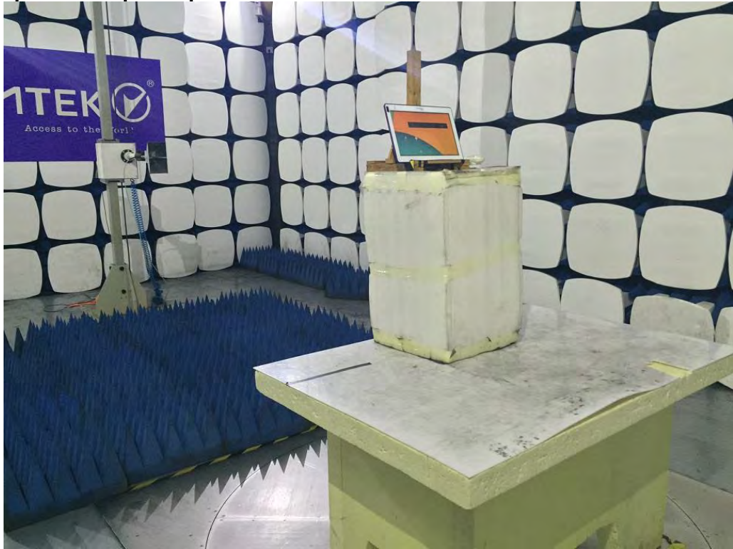
Photograph 4: Set-up for Spurious Emissions for 18 - 40GHz
