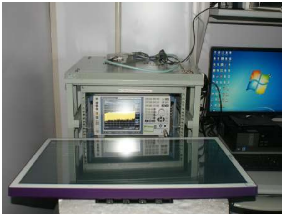
Photograph 1: Set-up for Radio Spectrum Test
