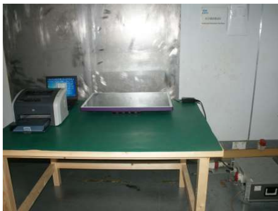
Photograph 6: Set-up for Conducted Emission on AC Mains
