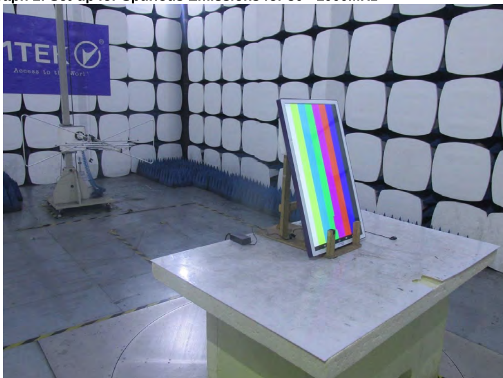
Photograph 2: Set-up for Spurious Emissions for 30 - 1000MHz
