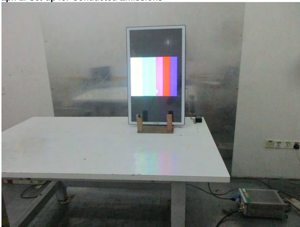
Photograph 2: Set-up for Spurious Emissions for 30 - 1000MHz
