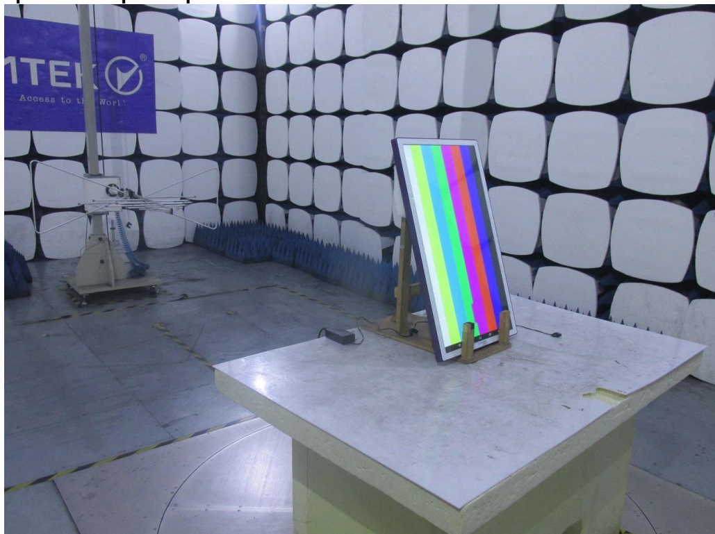
Photograph 2: Set-up for Spurious Emissions for 30 - 1000MHz
