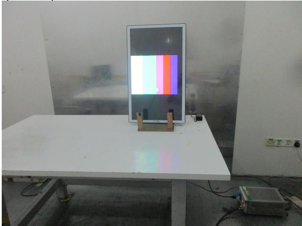
Photograph 2: Set-up for Spurious Emissions for 30 - 1000MHz
