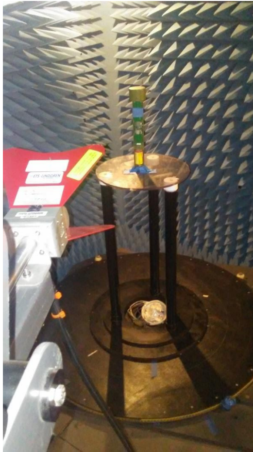
Photograph 4. Radiated Spurious Emissions, Above 1GHz, Test Setup
