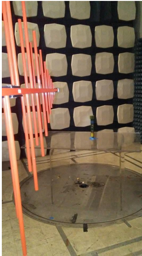
Photograph 3. Radiated Spurious Emissions, Below 1GHz, Test Setup
