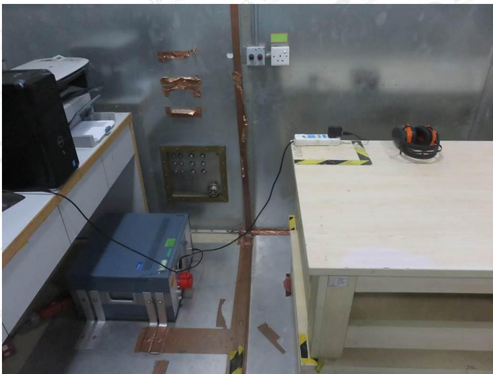
FCC RADIATED EMISSION TEST SETUP
