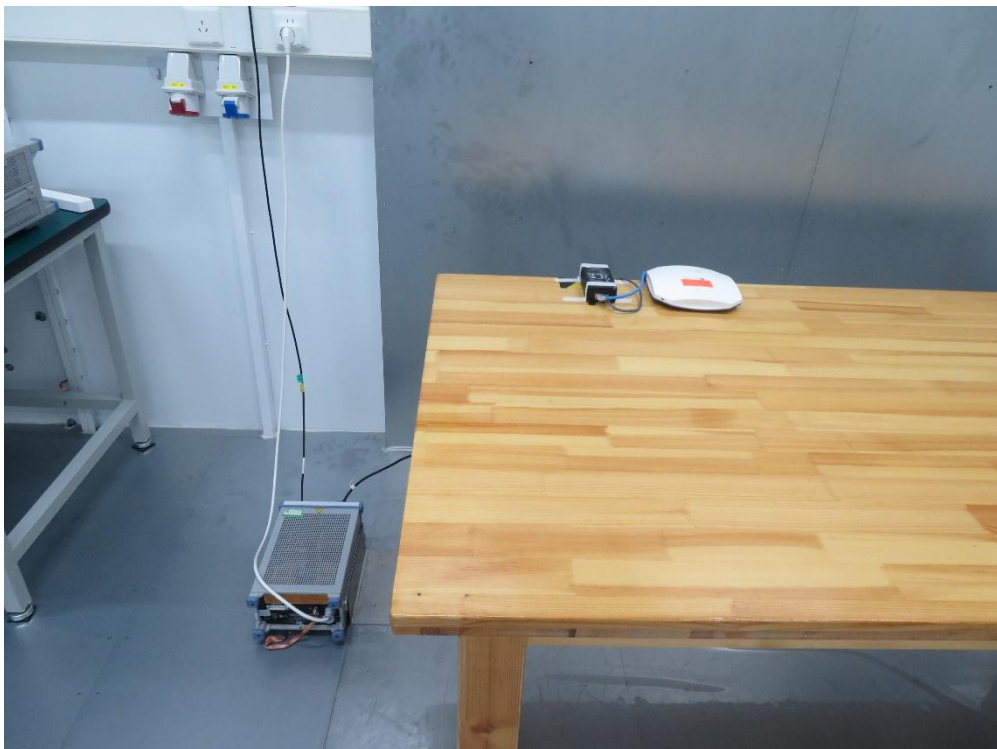
Description: Front View of Conducted Emission Test Setup (PoE Mode)
