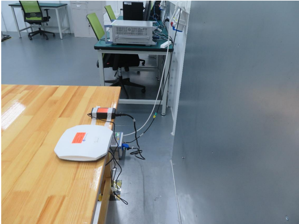
Description: Front View of Conducted Emission Test Setup (PoE Mode)
