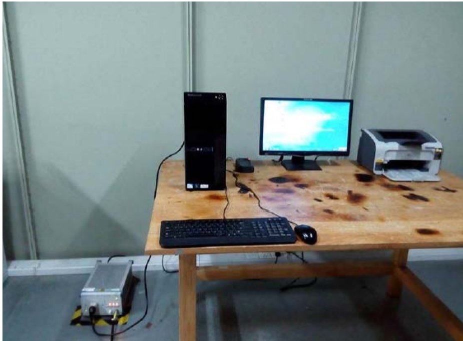
Conducted Emission Test Set-up –Front view
