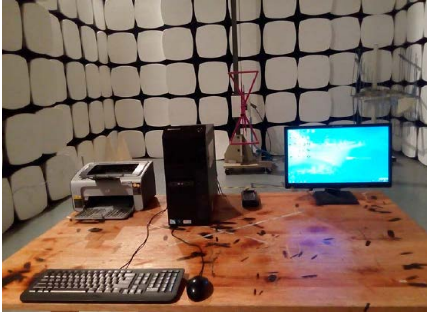
Radiated Emission Test Set-up(30-1000MHz)
