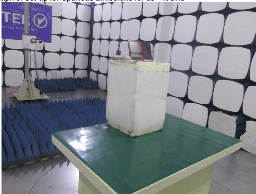
Photograph 3: Set-up for Spurious Emissions for 18 - 40GHz
