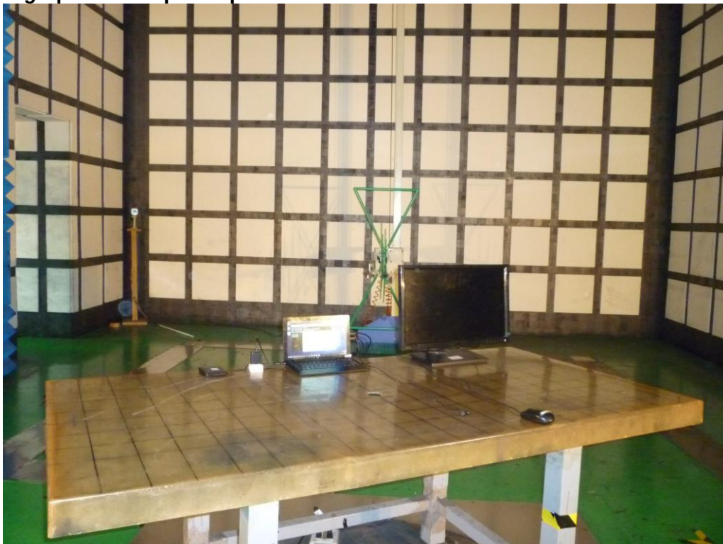
Photograph 2: Set-up for Spurious Emissions for 30 - 1000MHz
