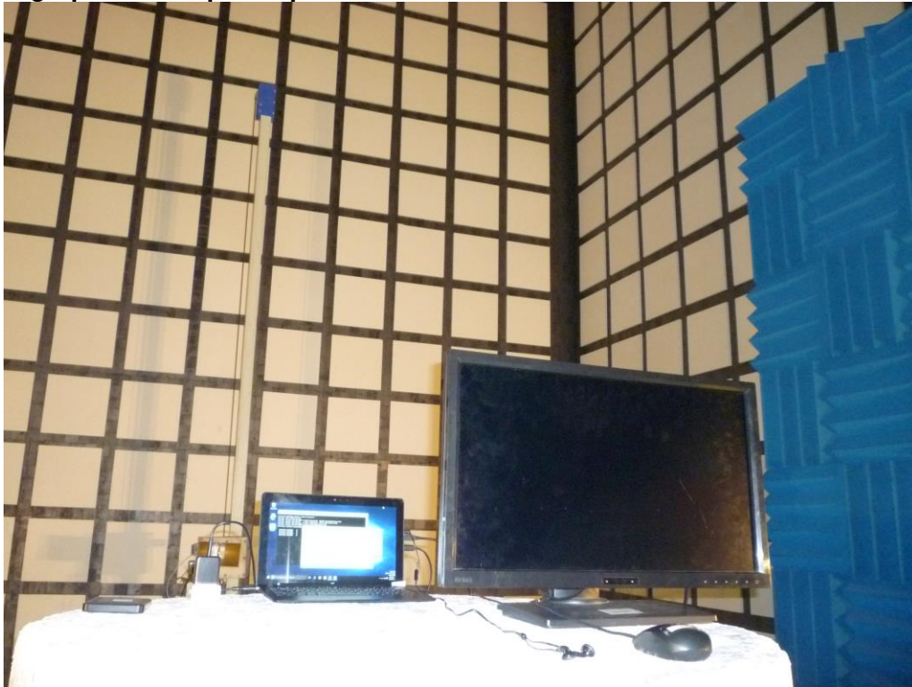
Photograph 3: Set-up for Spurious Emissions for 1 - 18GHz
