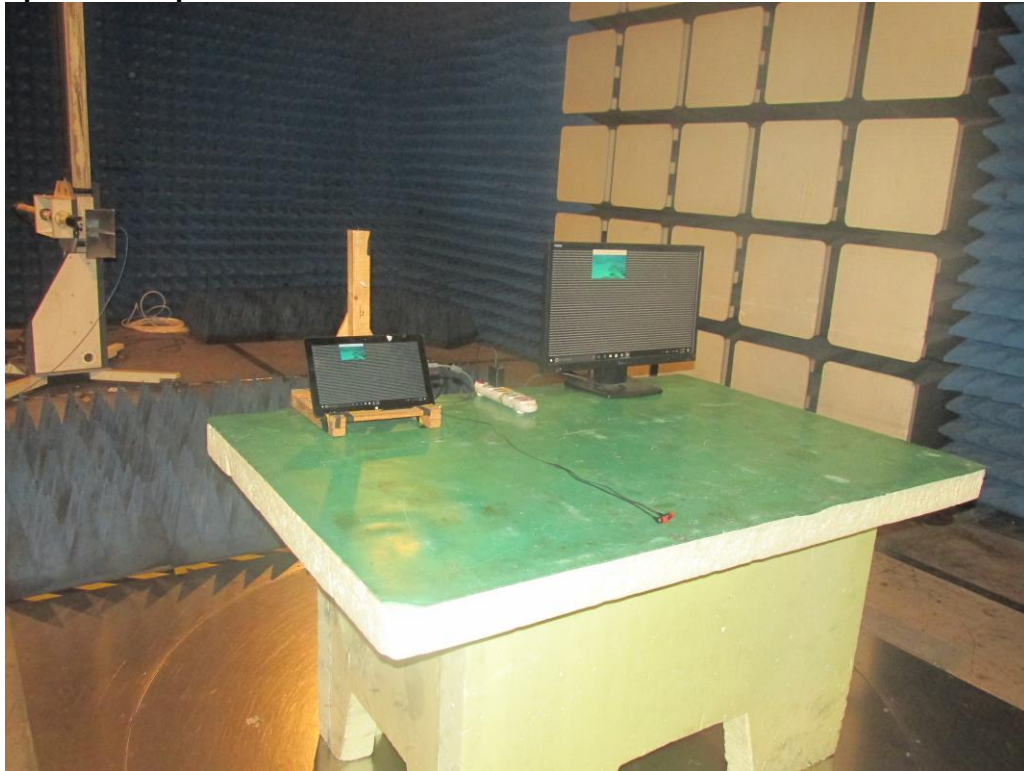
Photograph 3: Set-up for Radiated Emission of above 1GHz
