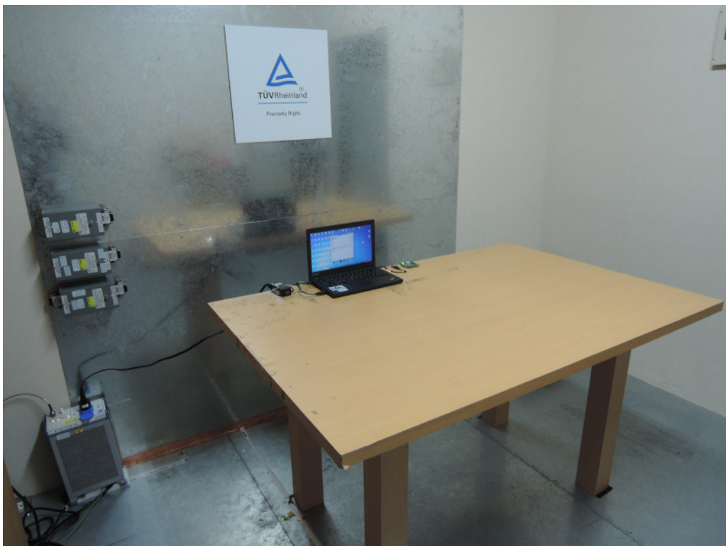
Photograph 7: Set-up for Mains Conducted testing (Front View)
