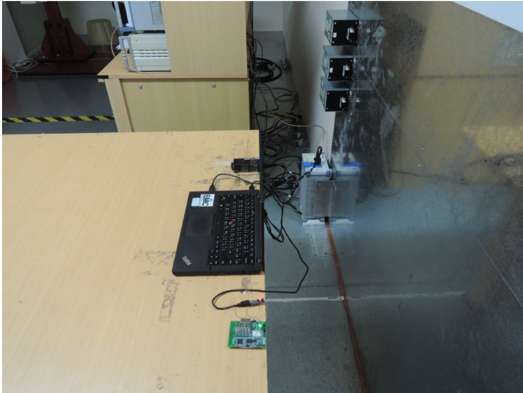
Photograph 6: Set-up for Mains Conducted testing (Back View)
