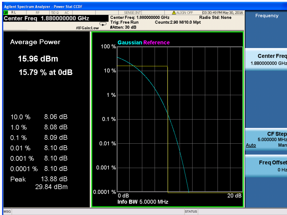
Peak-to-average power ratio plot on channel 810
