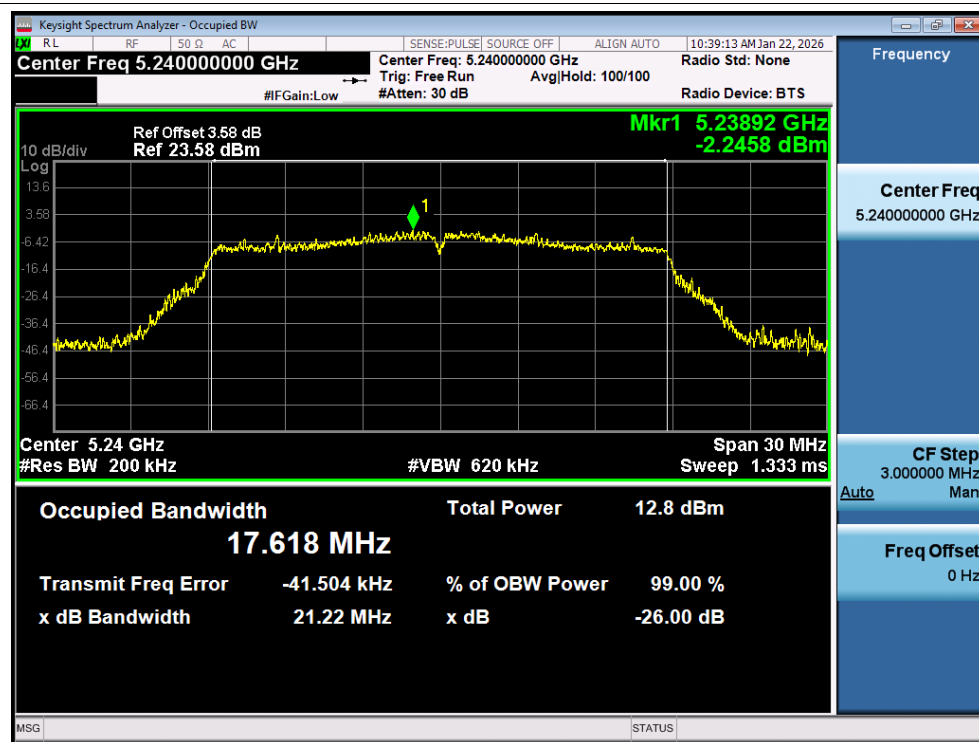
-26dB Bandwidth NVNT n20 5240MHz
