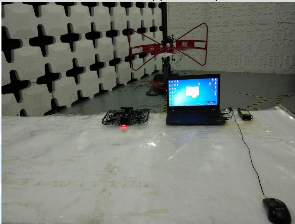
Radiated emission Test Setup (30 MHz~1 GHz) - Mode 4
