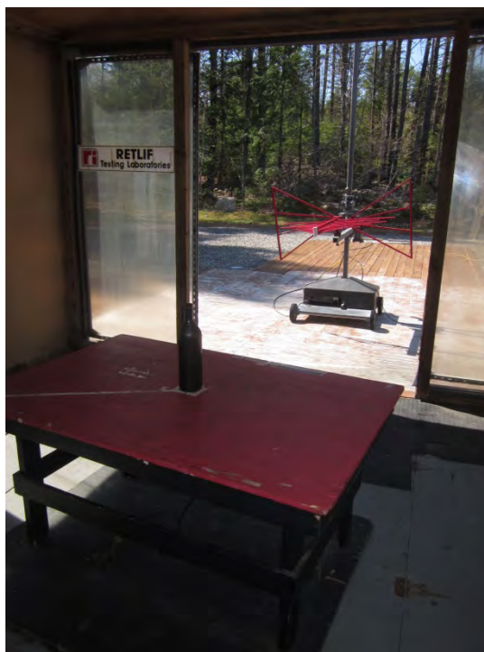
Test Setup, OATS, 30 MHz to 1 GHz, Horizontal Antenna Polarization
