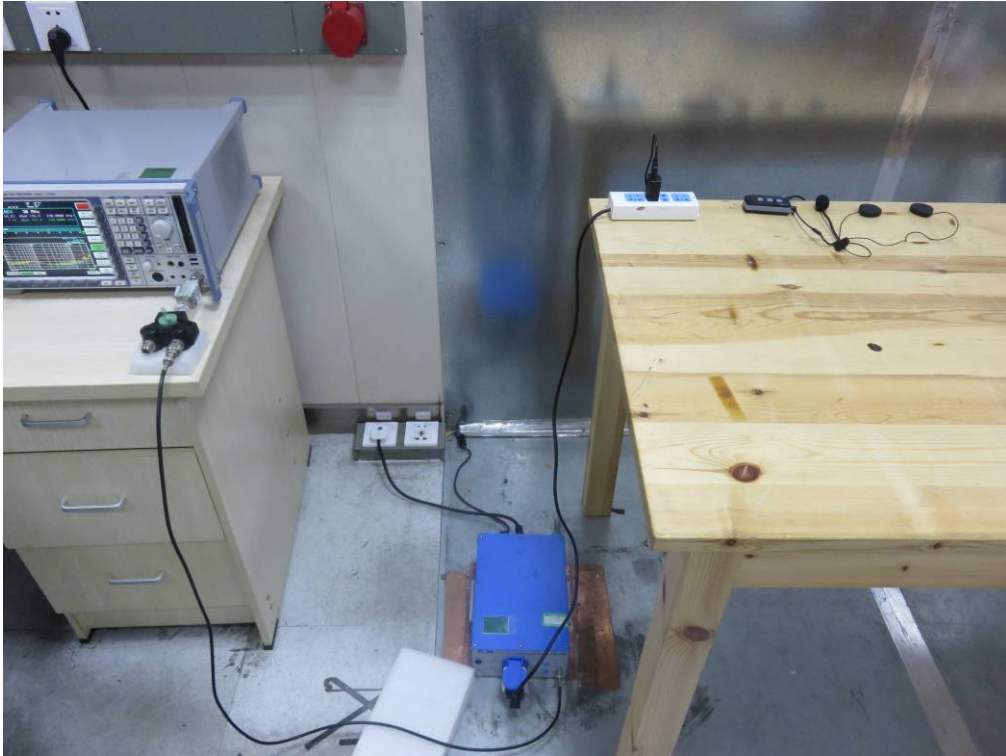
FCC RADIATED EMISSION TEST SETUP
