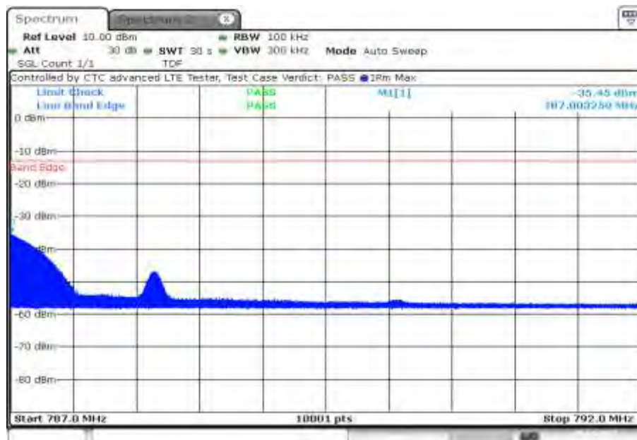
Plot 6: Highest channel, spacing 15 kHz, 1@0 tones
