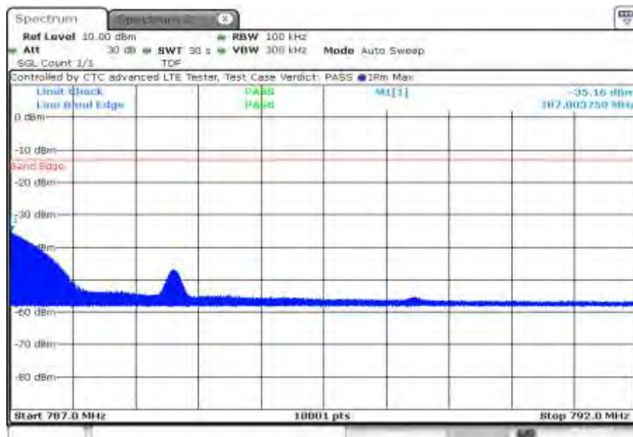
Plot 8: Highest channel, spacing 15 kHz, 1@11 tones
