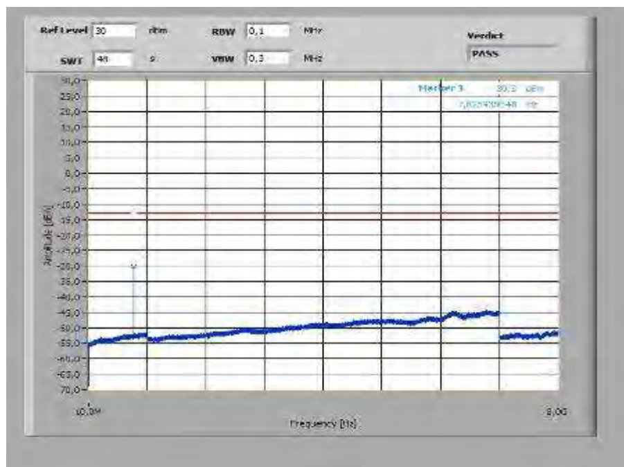
Plot 8: Middle Channel (10 MHz – 8 GHz), spacing 15 kHz, 1@0 tones
