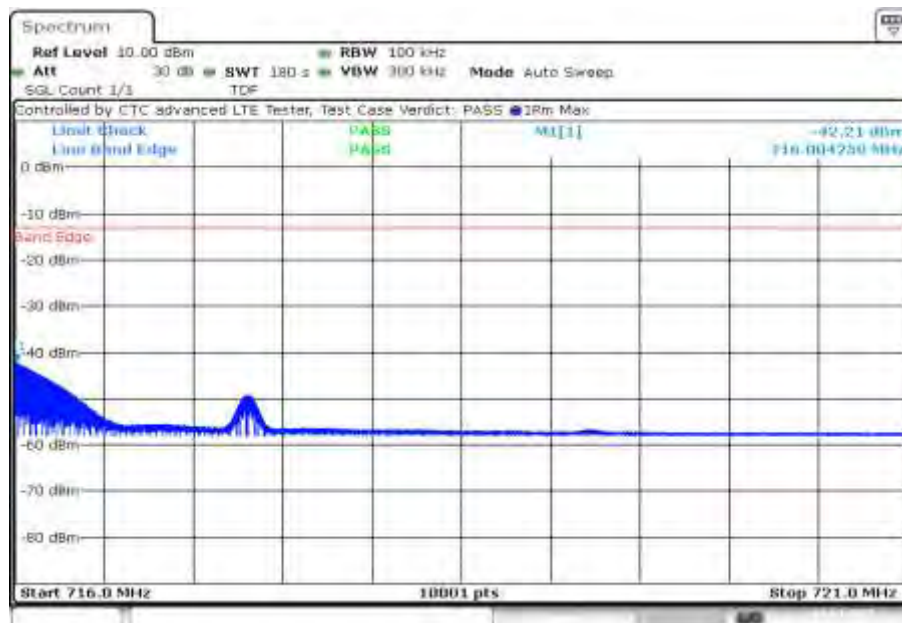
Plot 8: Highest channel, spacing 15 kHz, 1@11 tones
