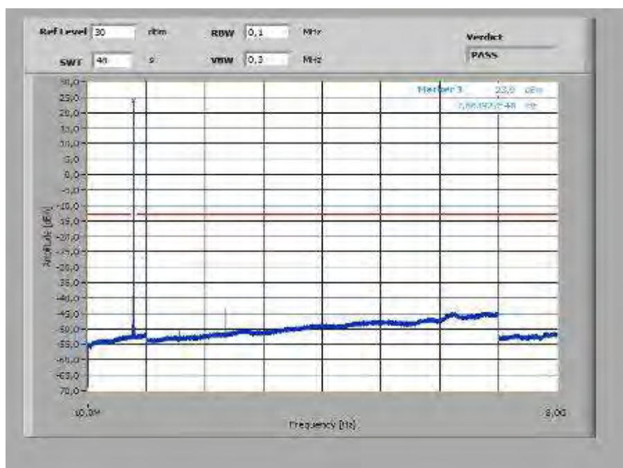
Plot 6: Highest Channel (10 MHz – 8 GHz), spacing 3.75 kHz, 1@47 tones
