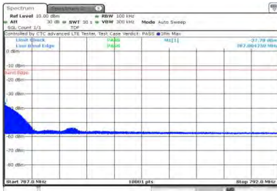
Plot 10: Highest channel, spacing 15 kHz, 12@0 tones
