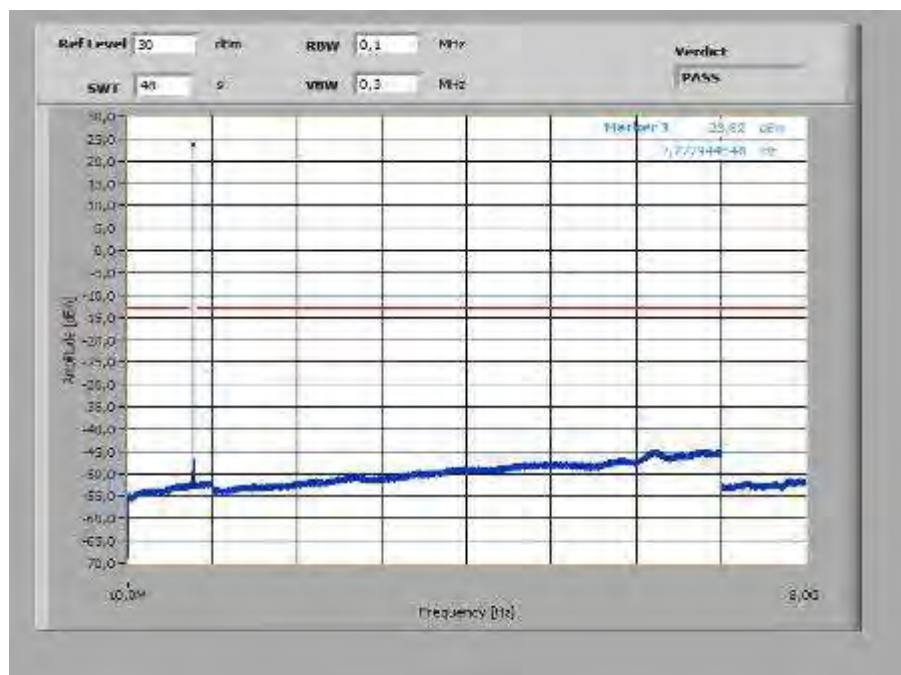
Plot 4: Lowest Channel (10 MHz – 8 GHz), spacing 3.75 kHz, 1@47 tones
