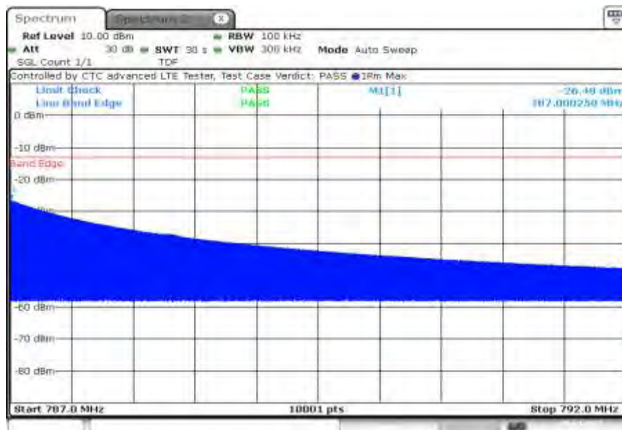
Plot 4: Highest channel, spacing 3.75 kHz, 1@47 tones
