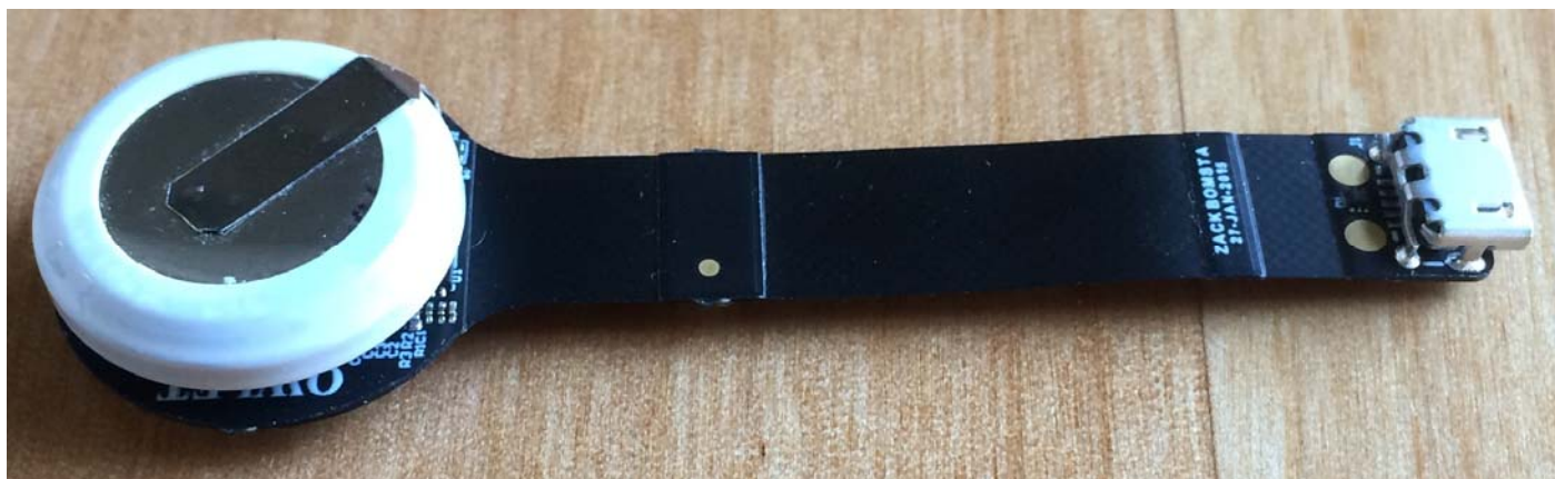
Figure 1 - Owlet Wearable Sensor - Showing Battery & Battery Clip
