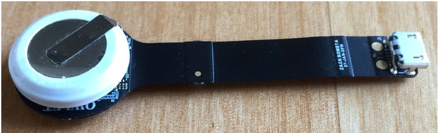
Figure 1 - Owlet Wearable Sensor - Showing Battery & Battery Clip
