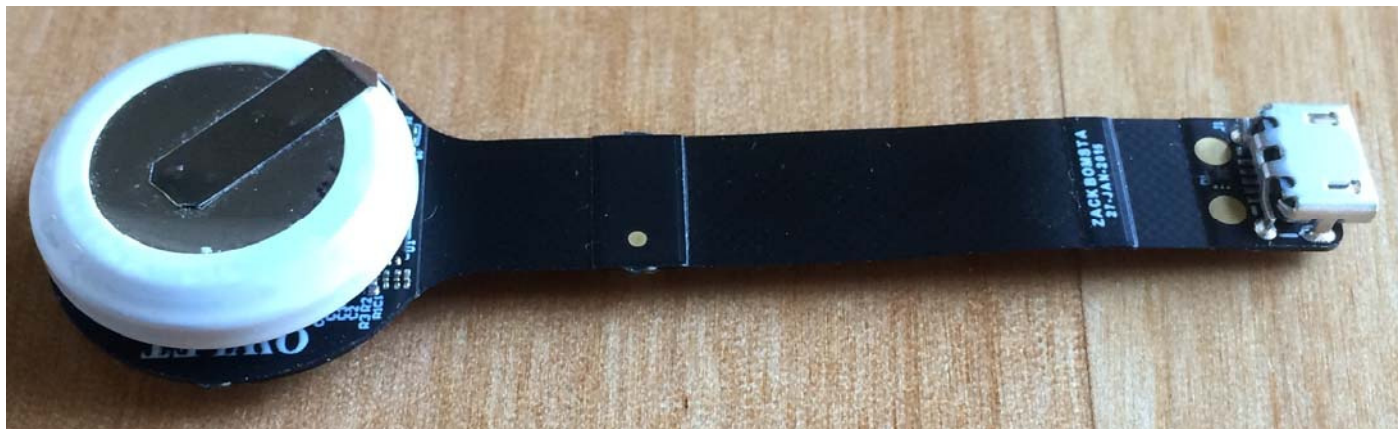
Figure 1 - Owlet Wearable Sensor - Showing Battery & Battery Clip
