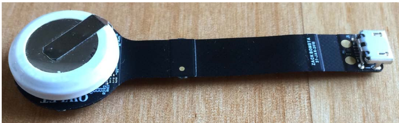
Figure 1 - Owlet Wearable Sensor - Showing Battery & Battery Clip
