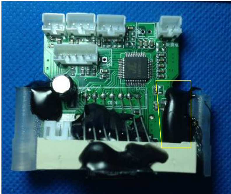
Internal BT Antenna Fixed in the PCB, 23mm, 1/5 wave
