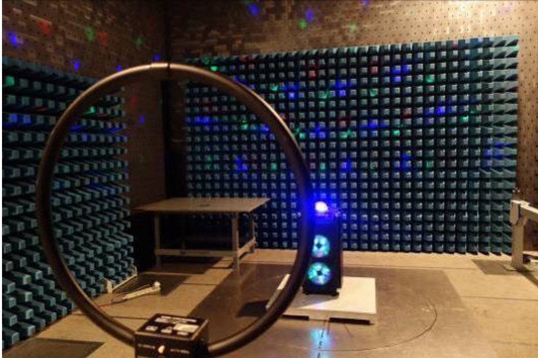
Re, Tested by Active Loop Antenna
