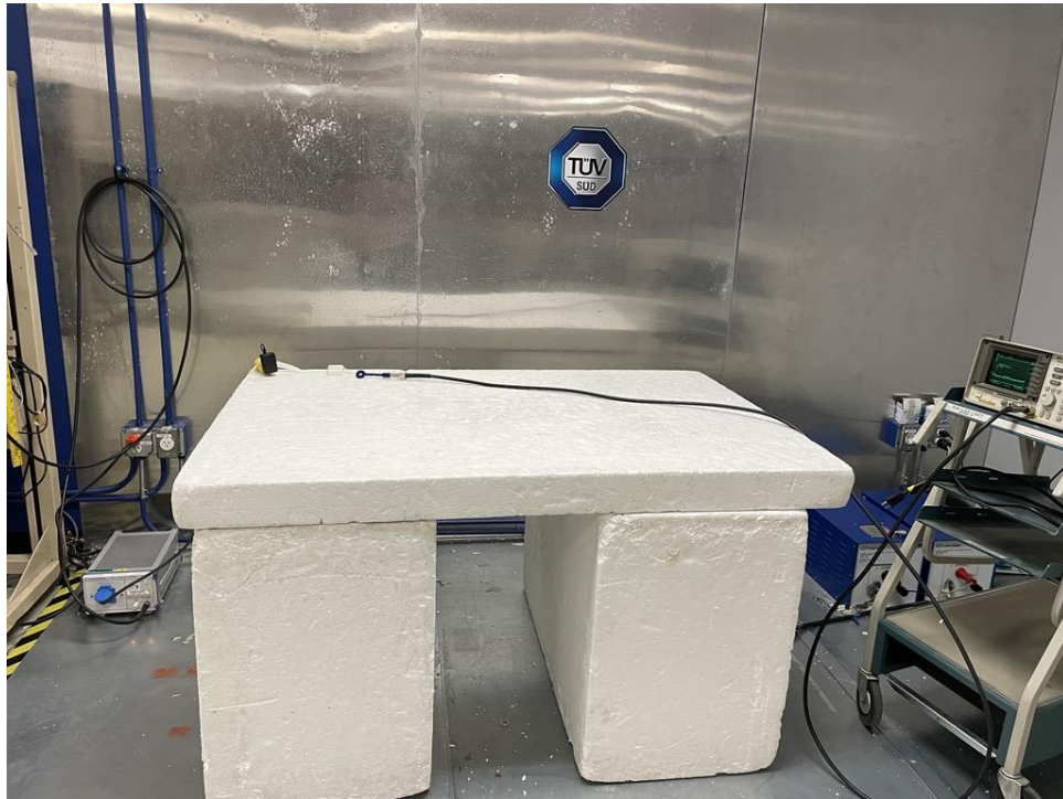
Figure 7– Test Set up – Conducted Emissions – 5V Power Supply
